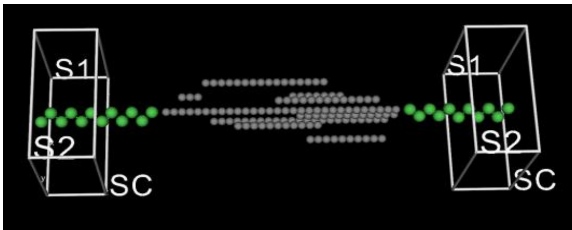
Figure 4.11: SWN composed of C monatomic wire plus 8 bonds between Ni electrodes ( p=0.5 ).
