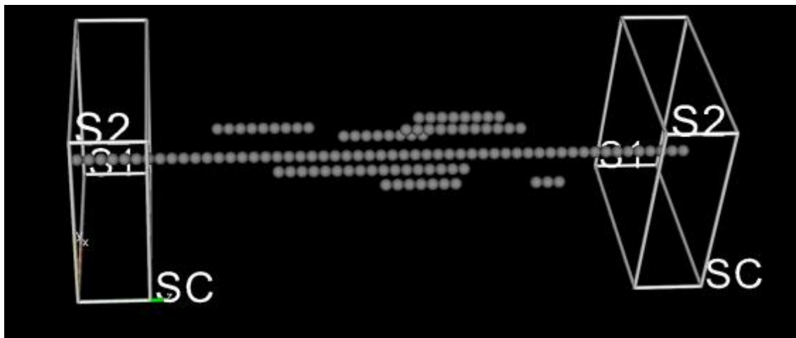
Figure 4.13: SWN composed of C monatomic wire plus 7 bonds between C electrodes ( p=0.2 ).
