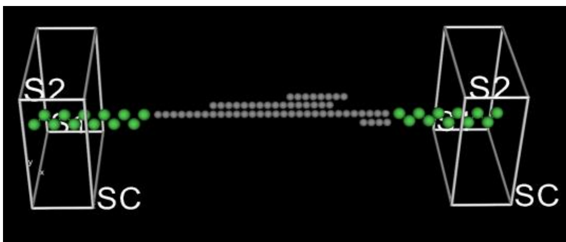
Figure 4.12: SWN composed of C monatomic wire plus 3 bonds between Ni electrodes ( p=0.1 ).
