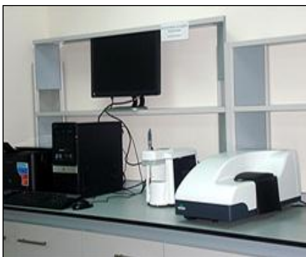
Figure III.14 Nano Sizer; Nano ZS, ZEN 3600 instrument.
