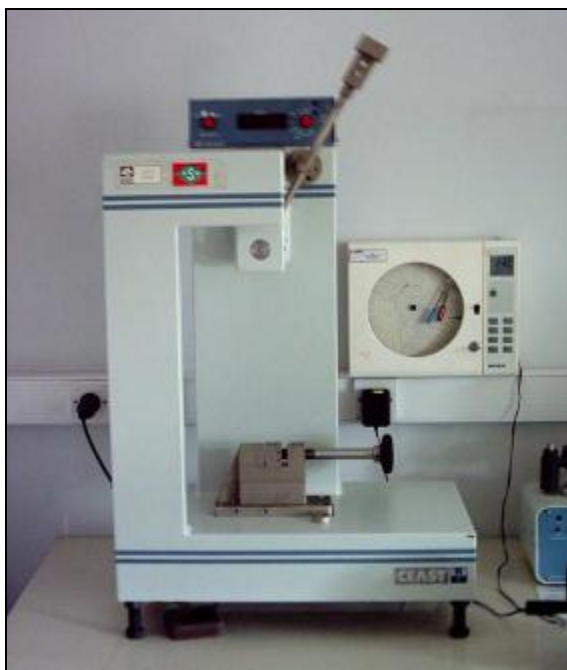
Figure III.19 Ceast impact tester.
