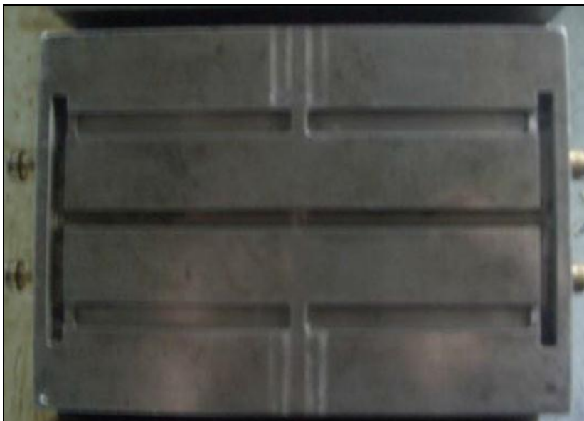
Figure III.11 Mold designs of Izod Impact test and LOI test specimens according to the ISO 180
