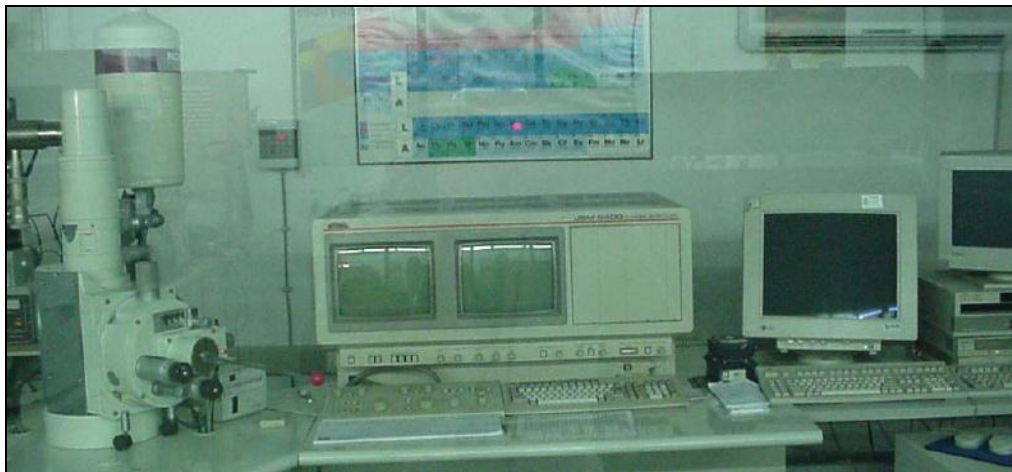
Figure III.16 JSM 6400 SEM ve NORAN Voyager EDS instruments.
