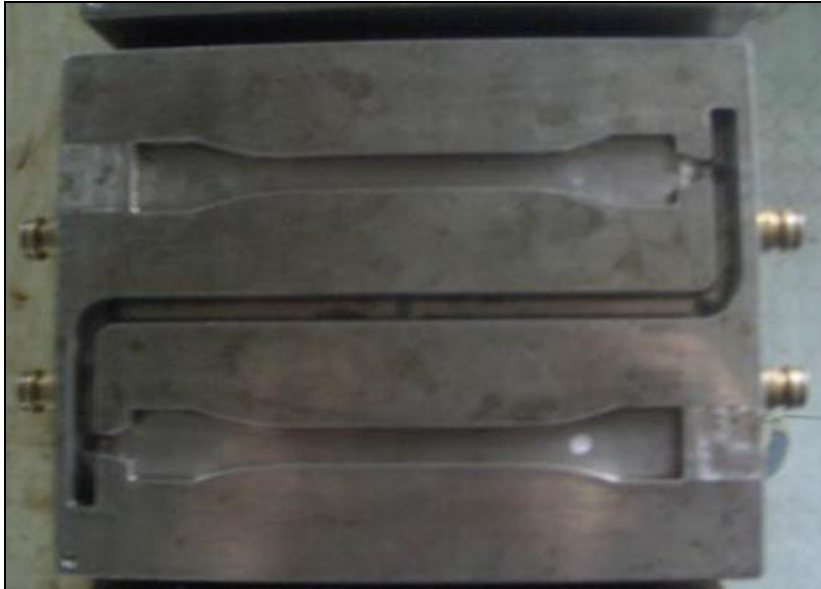
Figure III.10 Mold designs of tensile specimens according to the ISO R 527
