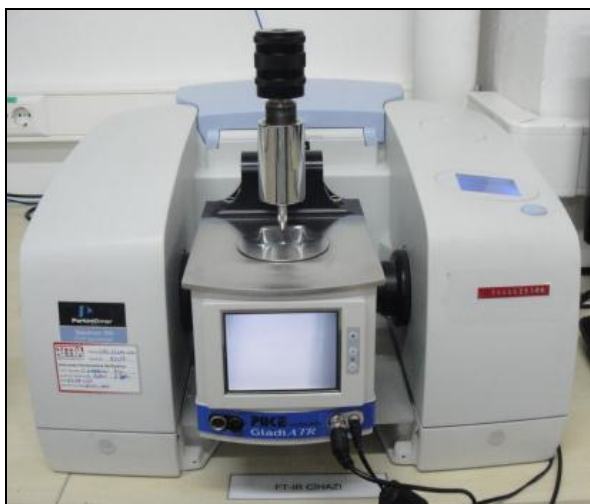
Figure III.13 Perkin-Elmer FT-IR Spectrum 100 spectrophotometer.
