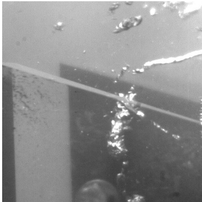
Figure 3.13: Near vertically oriented vortices in the shear layer between blocks (Frizell and Cox, 2009).
