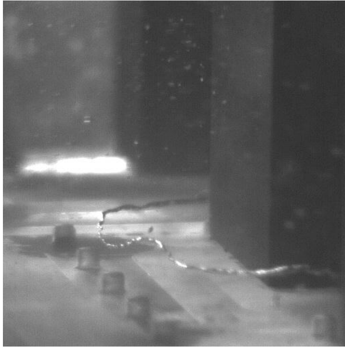
Figure 3.11: Horseshoe vortex upstream from baffle block face (Frizell & Cox, 2009)
