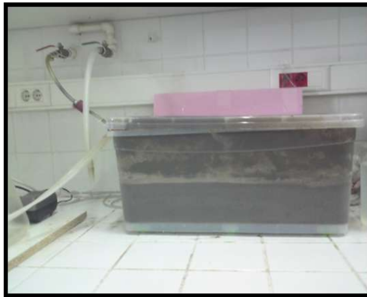
Figure 3.4. Picture of MBR set-up for domestic wastewater treatment
