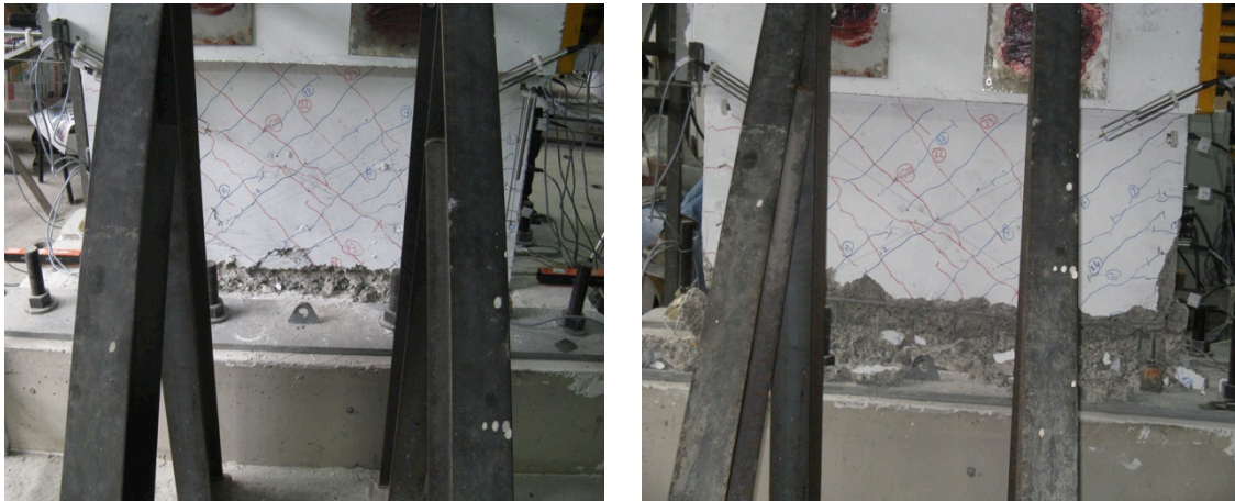
Figure 3.9. Medium and High Damage Levels (T2-S2).
