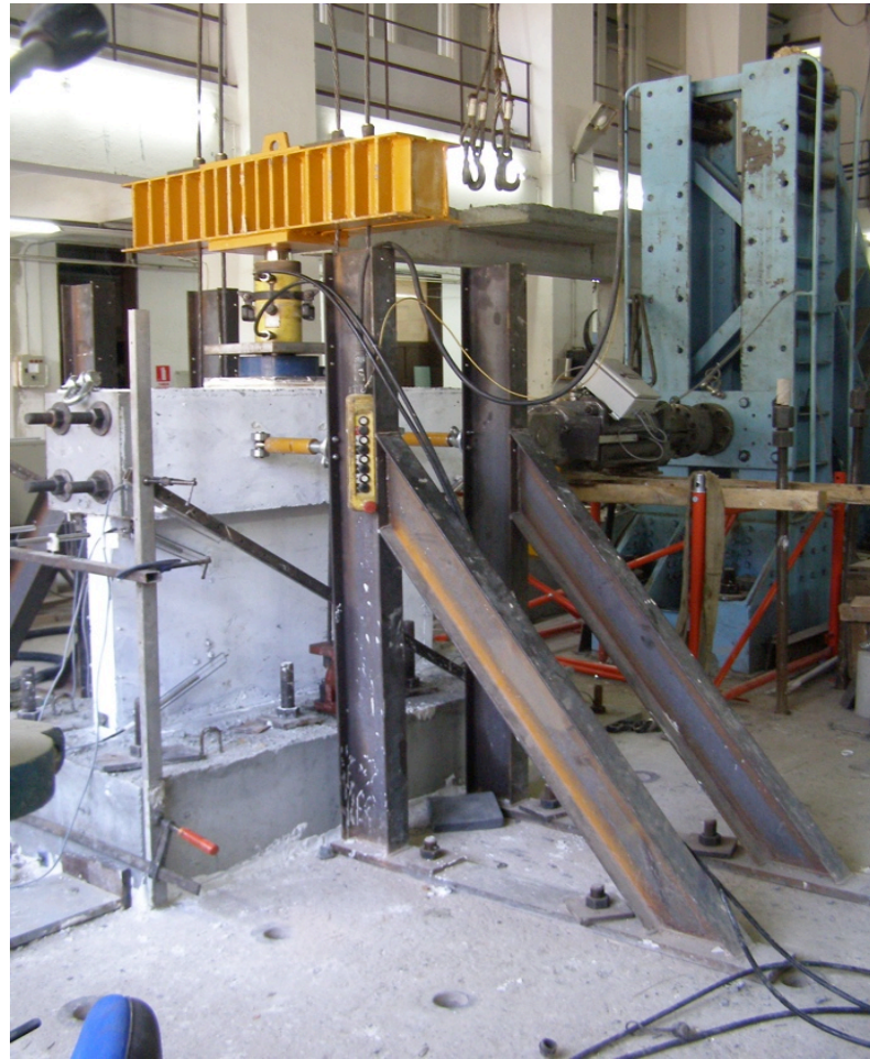
Figure 2.27. Axial Load Test Setup
