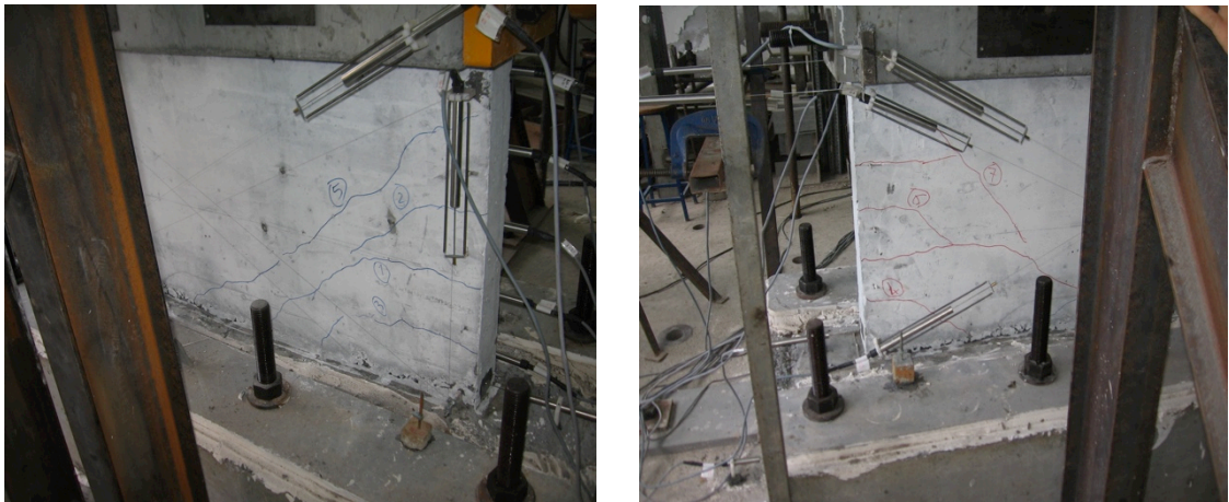
Figure 3.10. Initial Diagonal Cracks (T2-S3).
