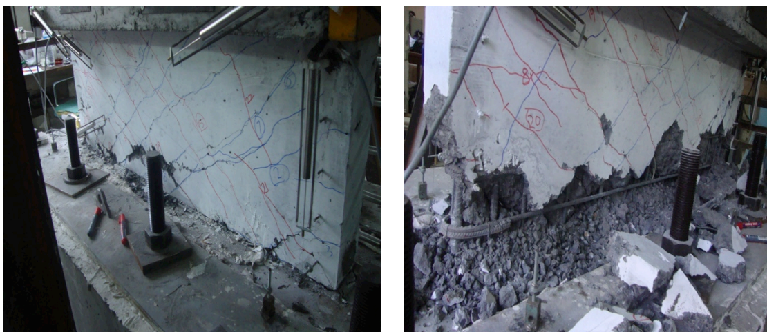
Figure 3.18. Medium and High Damage Levels (T4-S1).
