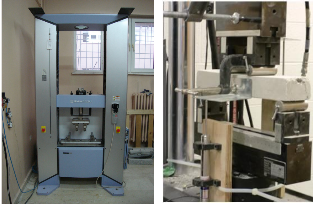
Figure 3.9. Four-point flexural strength test
