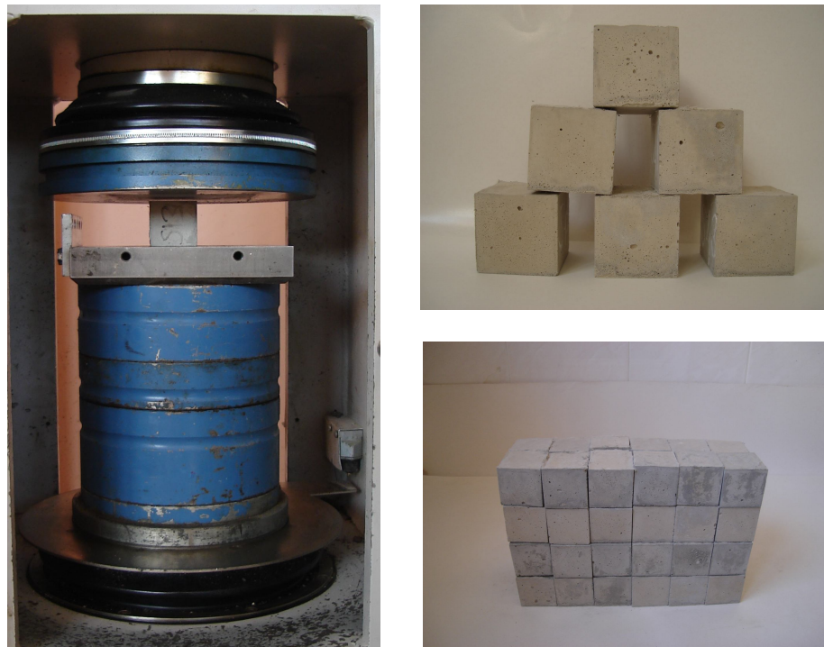
Figure 3.6 Compression testing machine and cubic samples
