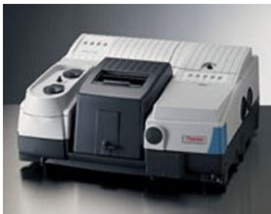
Figure 3.1 Nicolet 6700 FT-IR Spectrometer [57]
