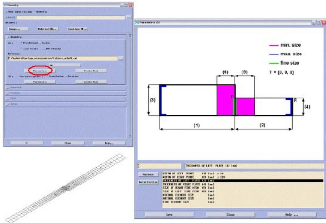
Figure 3.16. Heat source fitting tool.
