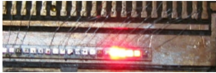
Figure 3.9. Different luminance values acquired using PWM.
