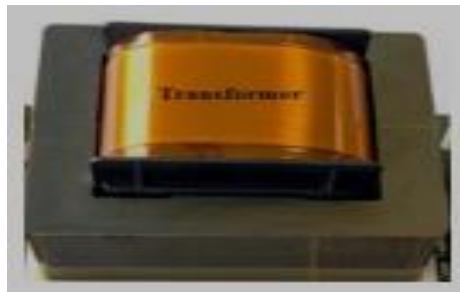
Figure 3.2. Conventional transformer winding. Image from Wikipedia.
