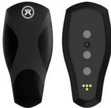
Resim 11: BSXinsight marka running model NIRS cihazı
