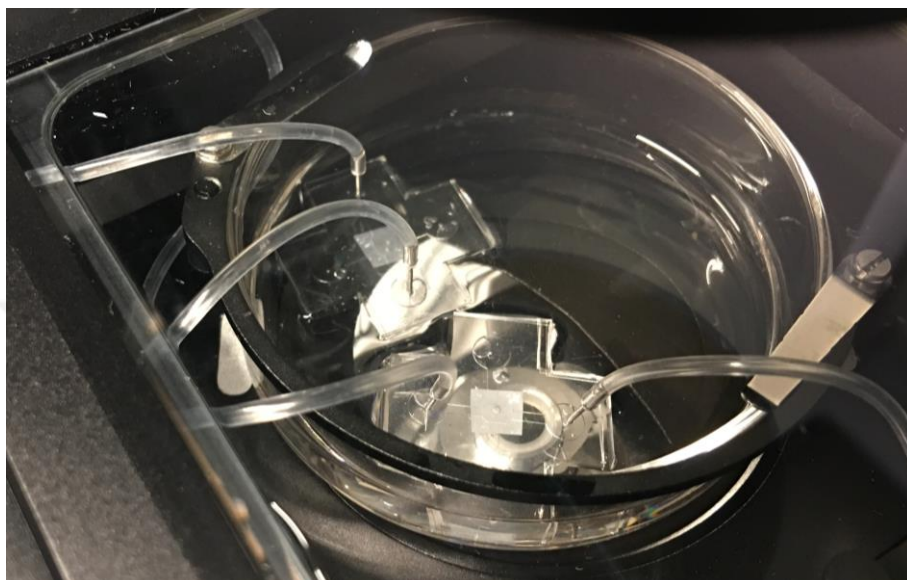
Figure 6.11 : Kidney-on-chip systems under static and dynamic conditions within the microscope stage top incubator system.
