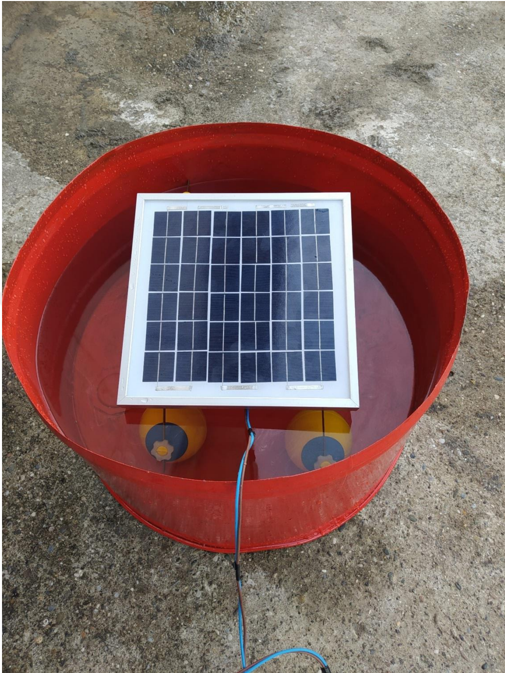
Figure 3.3. Installed solar panel floating on water.
