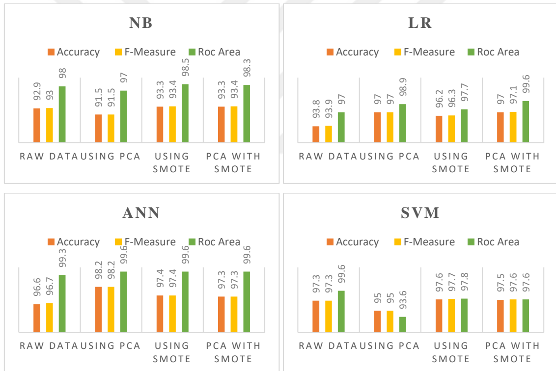
Figure 4.3. Performance of each classification algorithms for Dataset 3, before and after using (PCA, SMOTE, and PCA+SMOTE).
