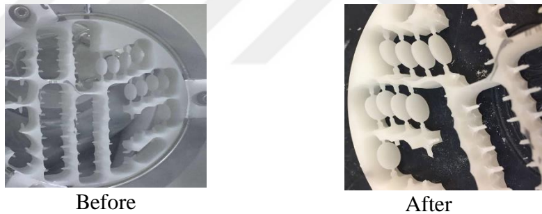
Figure 2: Before and after using the CAD/CAM milling machine to shape the wax disc
