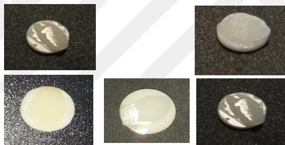
Figure 27: The final results of cementation different types of resin cements and material
