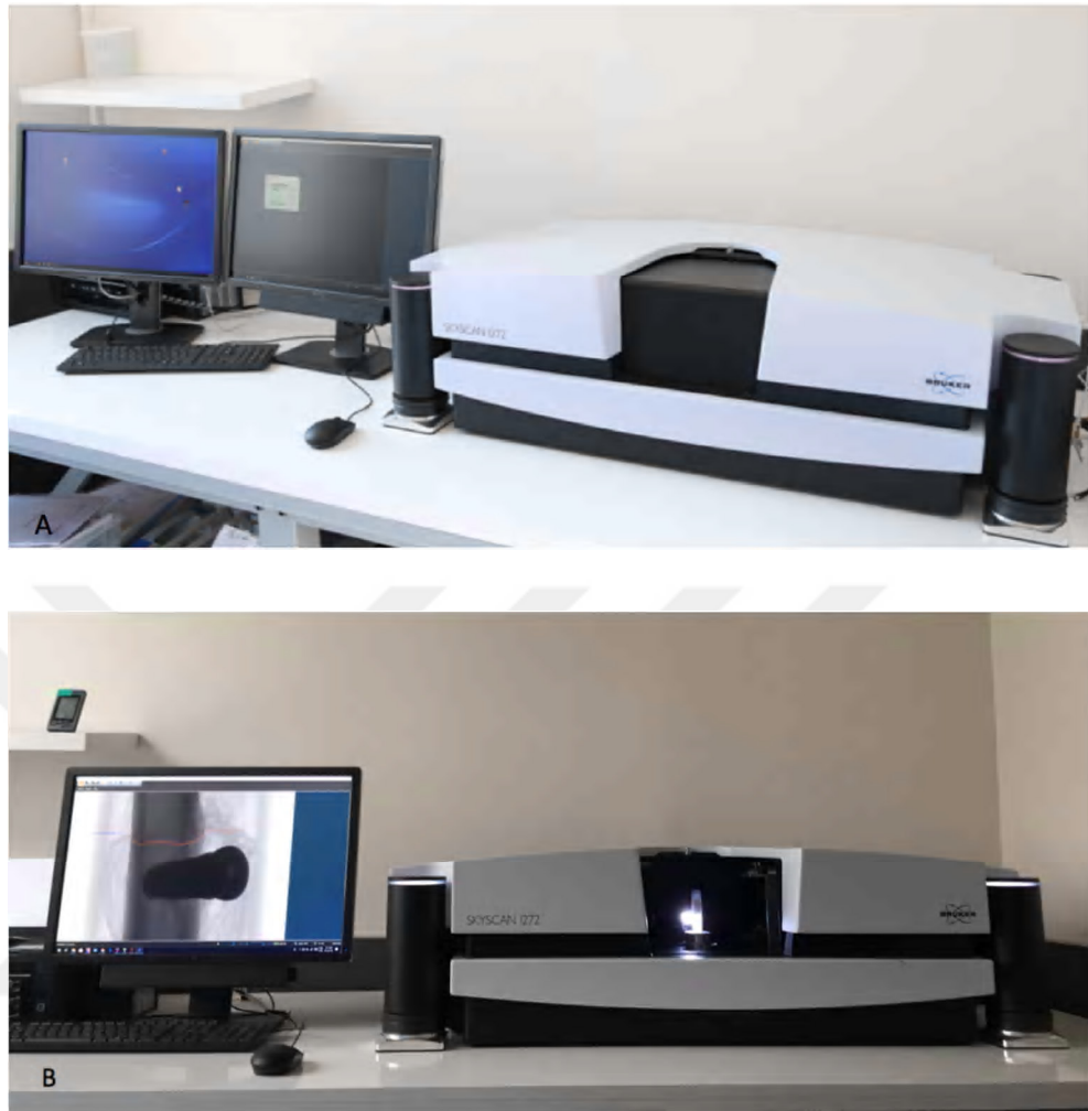
Figure 16. Skyscan 1272 Microcomputer Tomography device (A), Preparation of sample for scanning, insertion into device for scanning, scanning with device (B)
