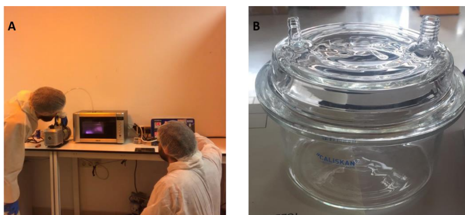
Figure 2.8 A. Air Plasma device. B. 8 mm thick borosilicate desiccator.
