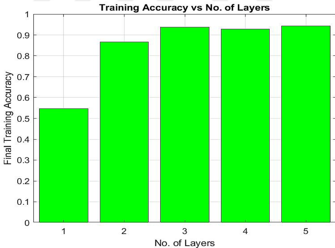
Figure 3.6. The training accuracy loss of ANN network with Spark Engine vs the number of layers.
