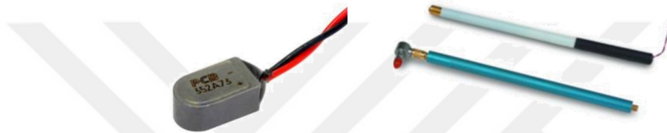
Figure 31 The Accelerometer and Impact Hammer for the Torquemeter Test
