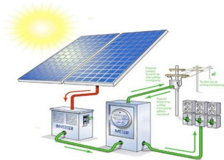
Figure 2.4: PV system working
