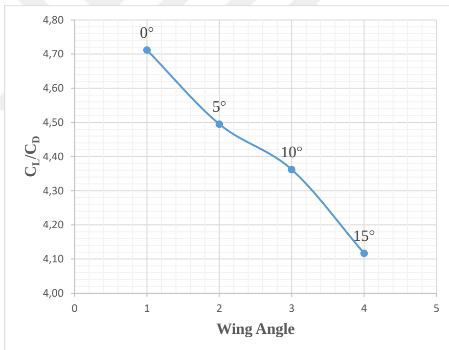
Figure 6.14 C_L/C_D ratio according to wing angle for 0° angle of attack
