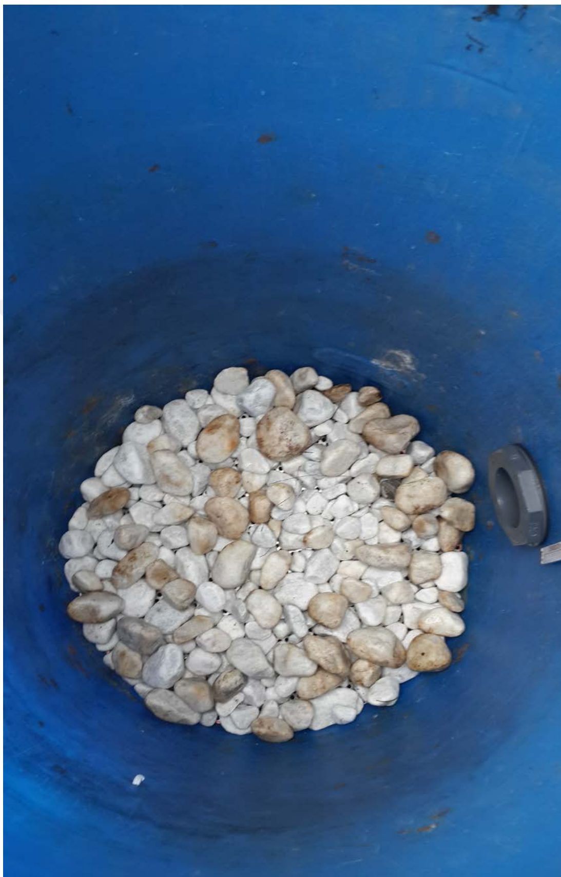
Figure 2.5 Stone layer of the compost reactor – Reactor I Germany (Personal archive, 2016)
