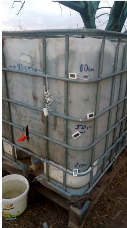
Figure 2.10 Position of the thermometers- Reactor III (Personal archive, 2020)
