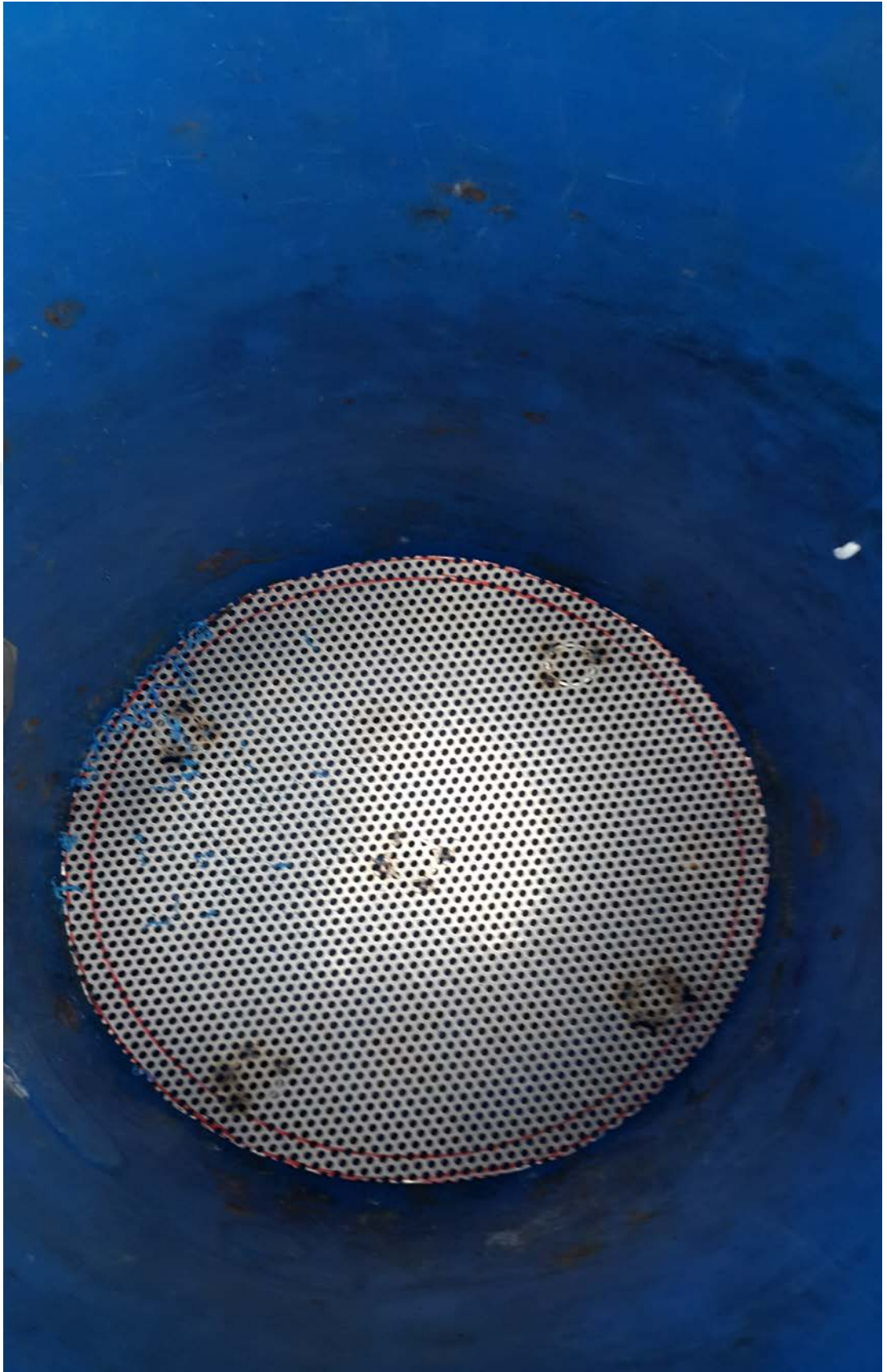
Figure 2.3 Compost reactor inside view/metal plate – Reactor I Germany (Personal archive, 2016)
