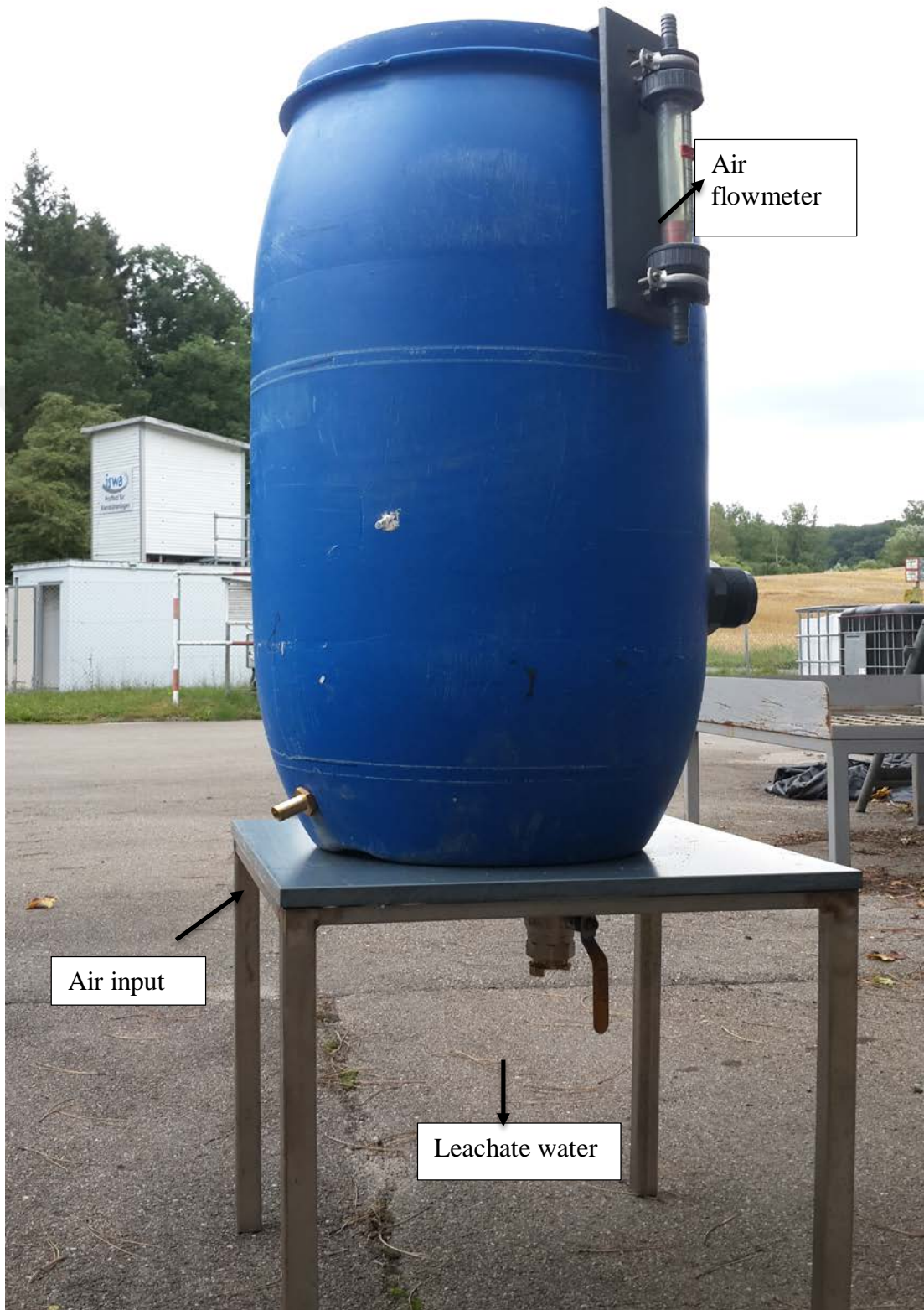
Figure 2.1 Compost reactor general view I- Reactor I Germany (Personal archive, 2016)
