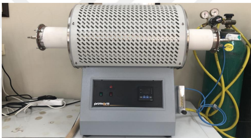
Figure 3.6 Atmosphere controlled furnace used in the carbonization
