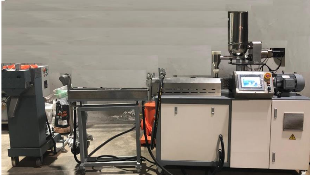
Figure 4.1 Twin screw extruder, water bath, and cutter/slicer used in the formation of frc-MB composites
