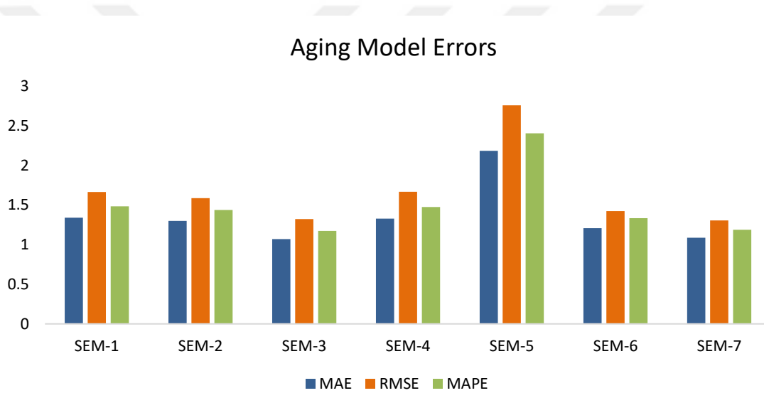
Figure 21. Performance indicators for each LFP dataset modeling with GA.
