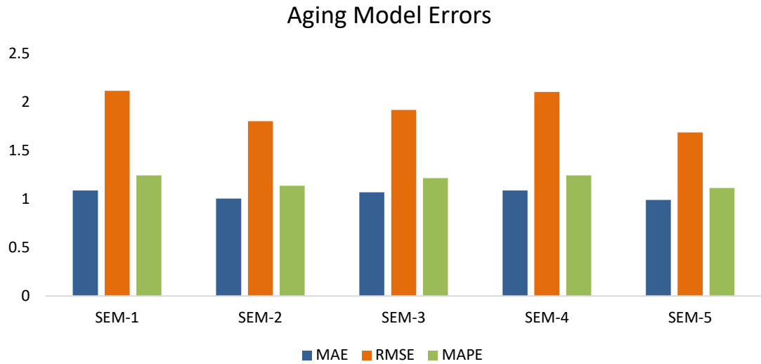
Figure 18. Performance indicators for each NMC-2 dataset modeling with analytical solution.
