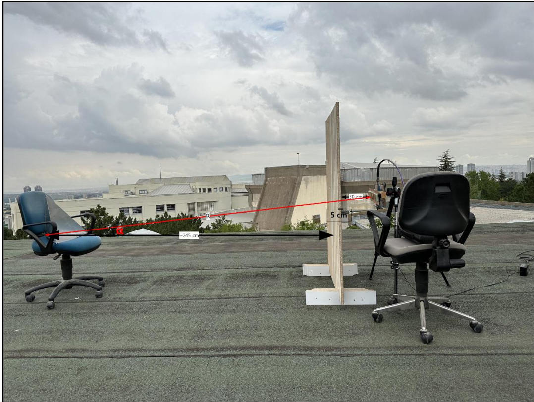
Figure 6-10 TWR Setup-3, target is placed to the plywood as distance of around 245 cm.
