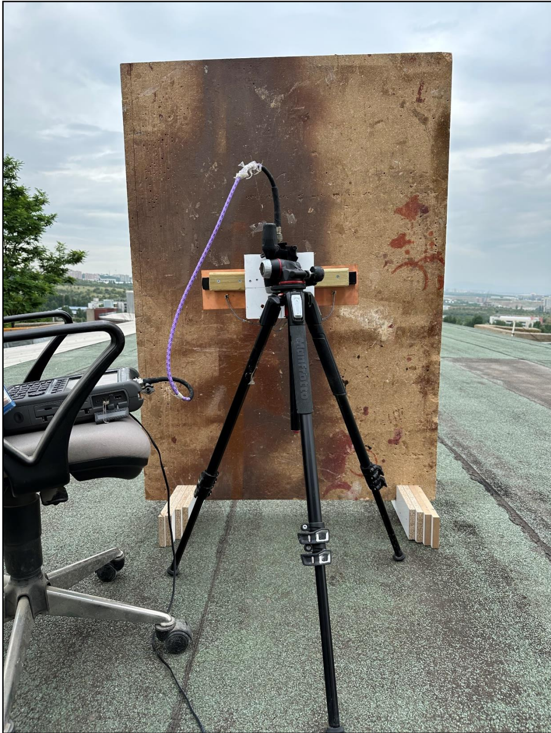
Figure 6-3 Photo-2 of experimental TWR setup with E-patch antenna array.
