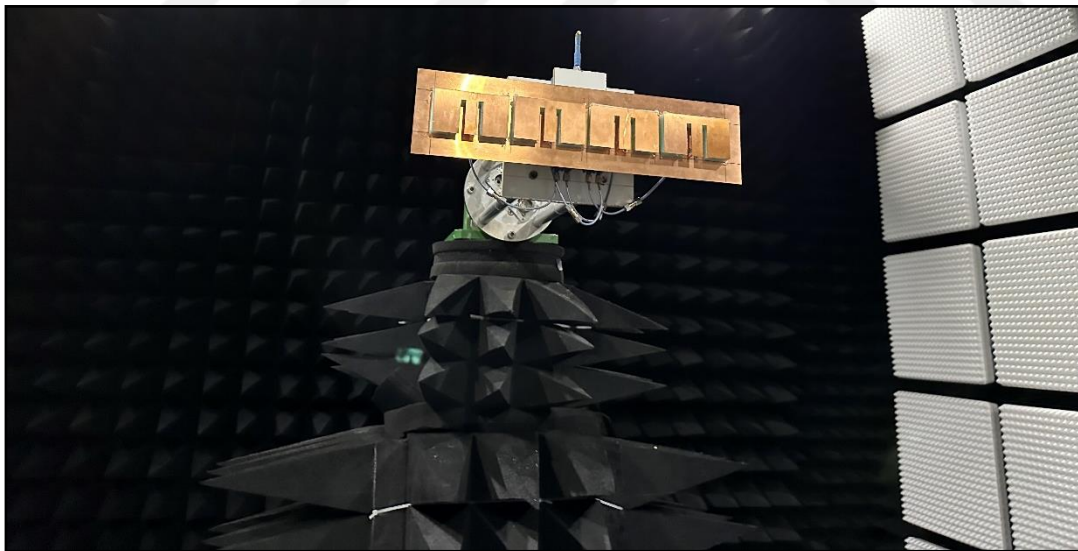
Figure 5-16 Photo-2 of manufactured E-Patch antenna array for azimuthal (H-Plane) radiation pattern measurements in METU EEE Anechoic Chamber.
