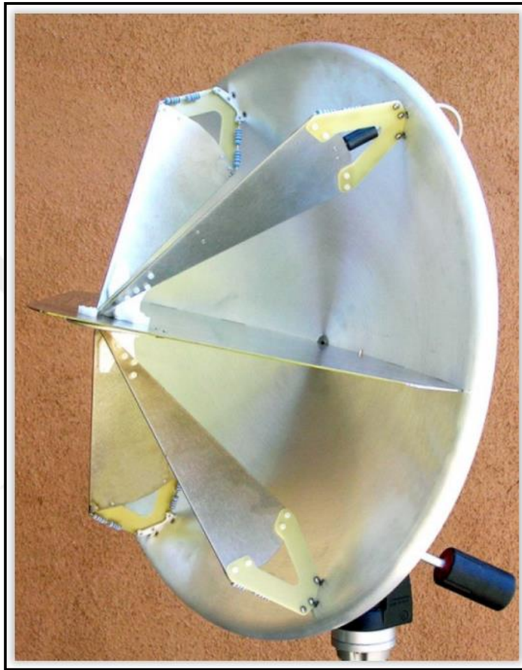
Figure 1-8 IRA-3Q operates from 250 MHz to 18 GHz and has a time response of fewer than 100 picoseconds [18].
