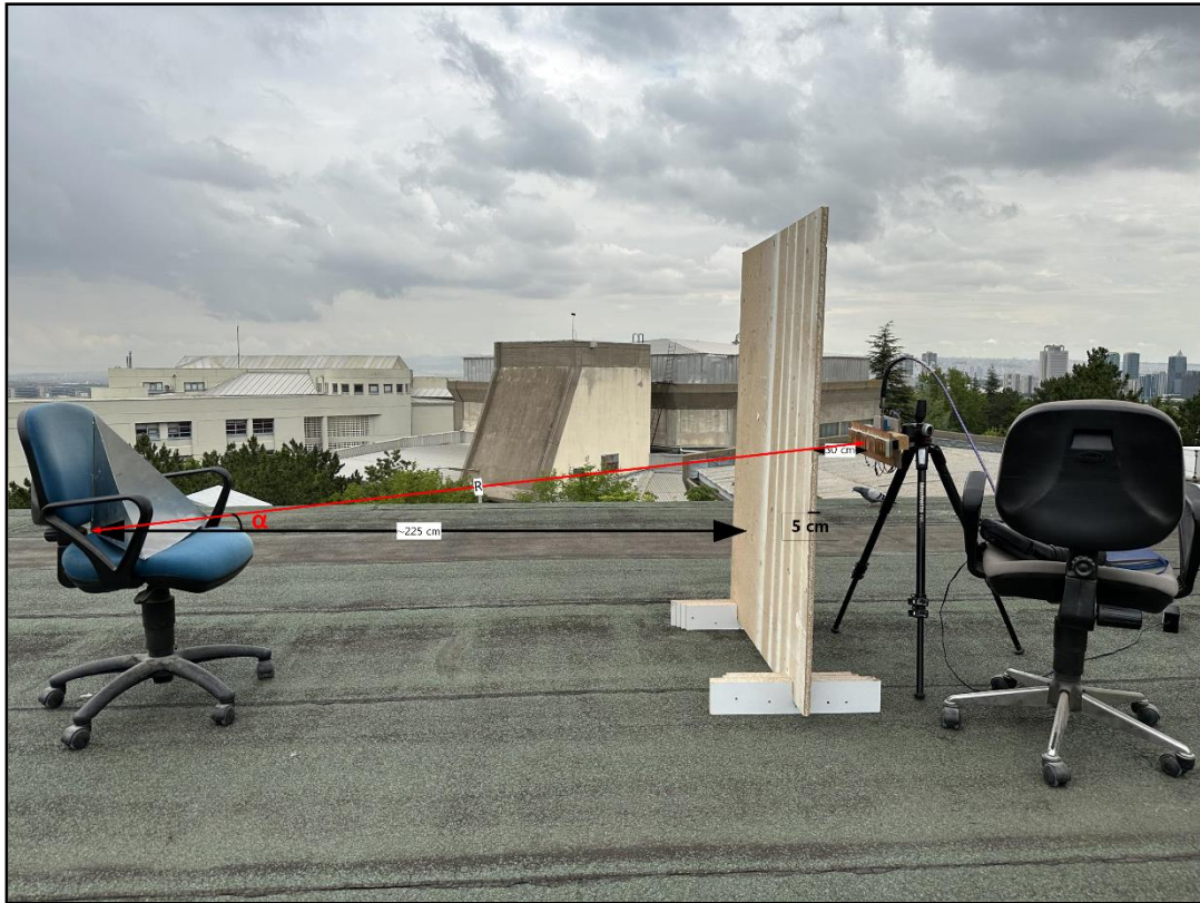
Figure 6-8 TWR Setup-2, target is placed to the plywood as distance of around 225 cm.
