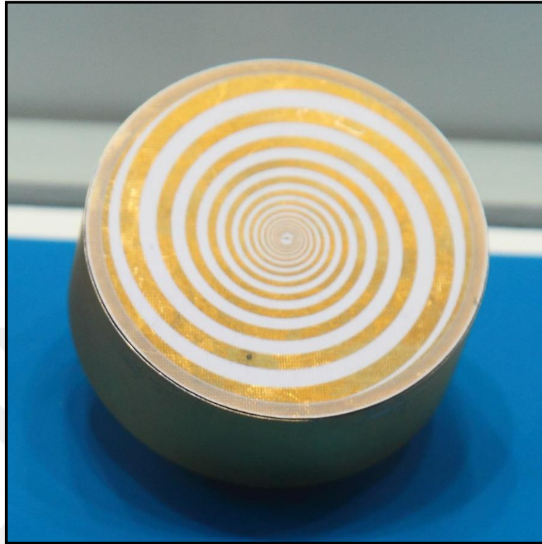
Figure 1-11 Two-arm, tightly wrapped, the logarithmic spiral antenna [34].
