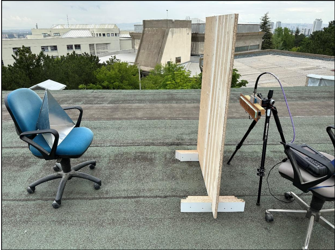
Figure 6-2 Photo-1 of experimental TWR setup with E-Patch antenna array with a corner reflector as the target object.
