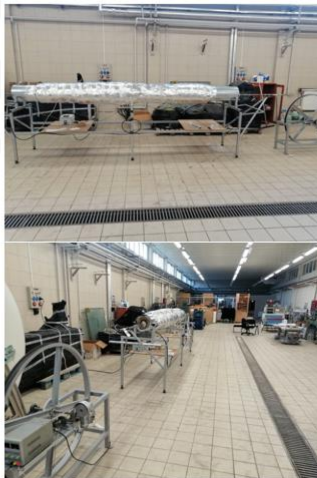
Figure 4.3. The photos of long tube furnace used for the intermediate heat treatment.
