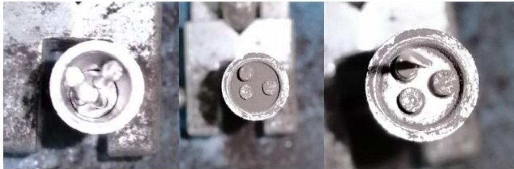
Figure 4.8. The photos show each step during the filling process of the TH-IMD method.
