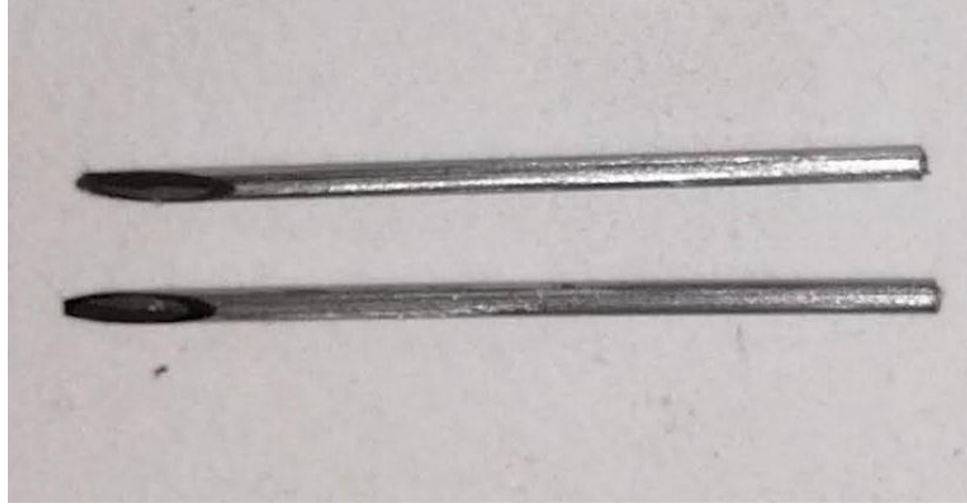
Figure 4.15. Picture of unreacted \text{MgB}_2 wires with 15^\circ angled ends.
