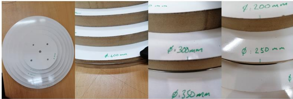
Figure 4.26. Circular apparatus used to bend \text{MgB}_2 wire pieces. Each disc has a different diameter.
