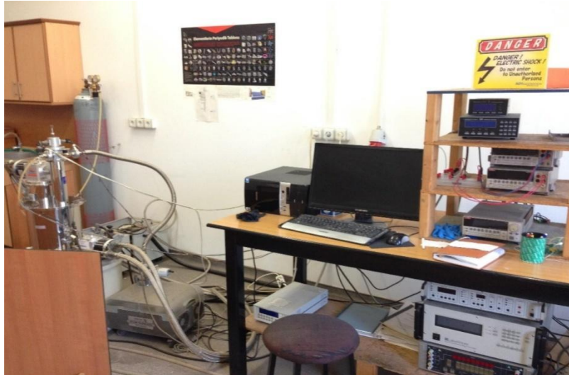
Figure 4.22. Closed cycle cryostat system with 7 T superconducting magnet used for transport measurements.
