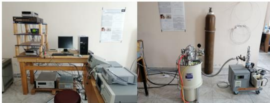
Figure 4.23. Closed cycle cryostat system with 4.5 T superconducting magnet used for transport and magnetic field decay measurements.
