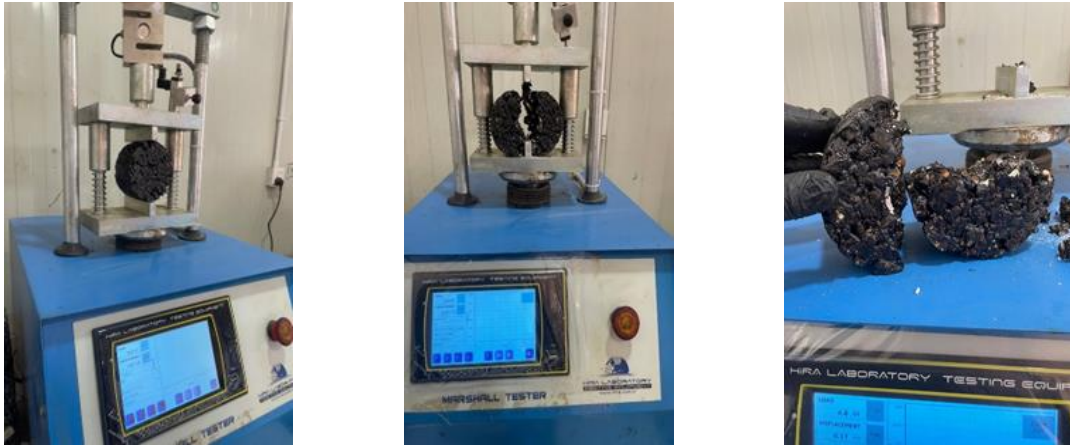
Figure 3.8: Instrument for Indirect Tensile Strength Testing (2003b).
