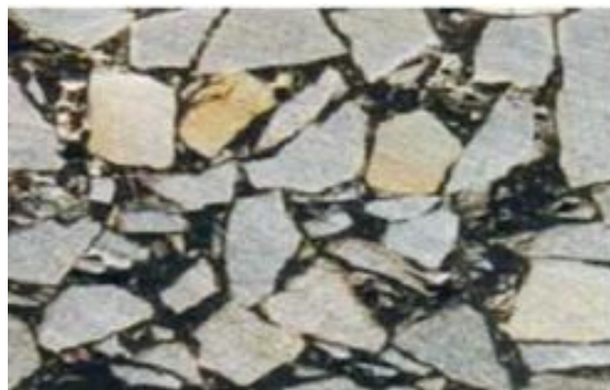
Figure 1.1: Depicts the Cross-Sectional View of Stone Mastic.
