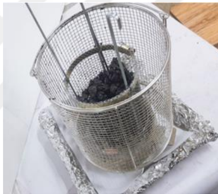
Figure 3.6: Configuration of the Basket and Sample for the Drain Down Test.
