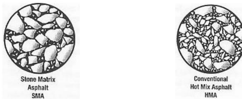
Figure 2.3: Illustrates Contrasts Between SMA and Traditional HMA.
