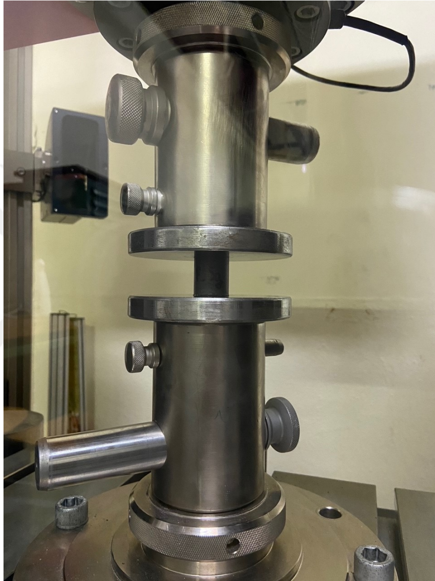
Figure 2.15: Uniaxial compression test setup
