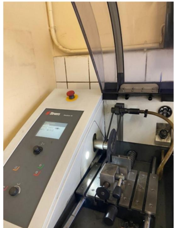
Figure 2.3: Waterjet (left) and metallographic cut-off machine (right)
