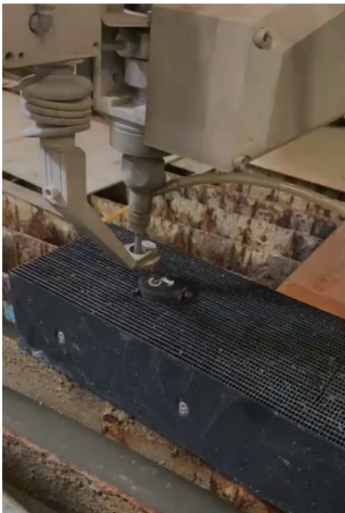
Figure 2.3: Waterjet (left) and metallographic cut-off machine (right)
