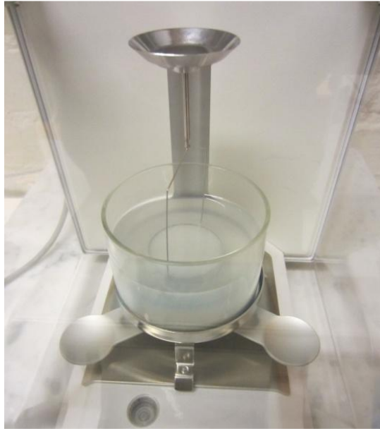
Figure 1.8 The set-up used for measuring the sedimentation rate of Nanofluids
