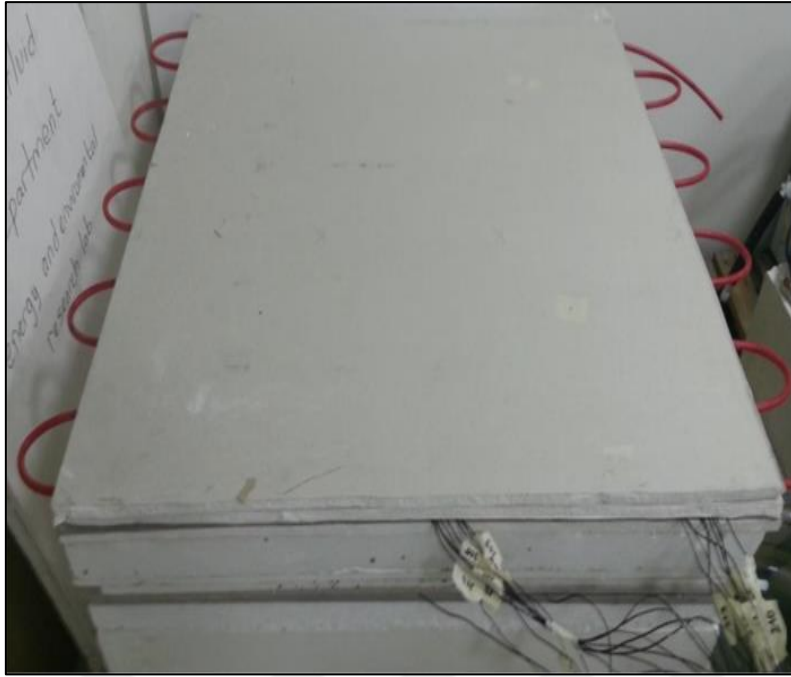
Figure 3.14 Heat transfer layer placed on the hybrid wall specimen.
