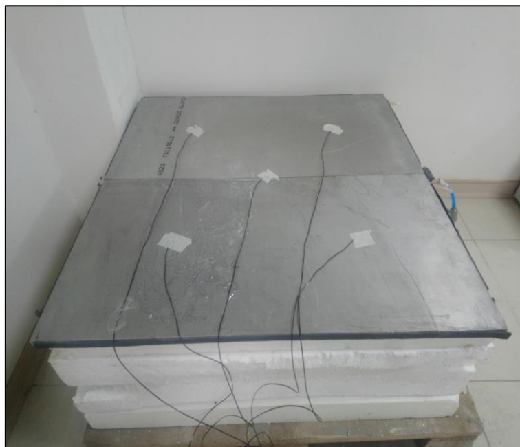
Figure 3.12 Cooling plate and thermocouples placed on it
