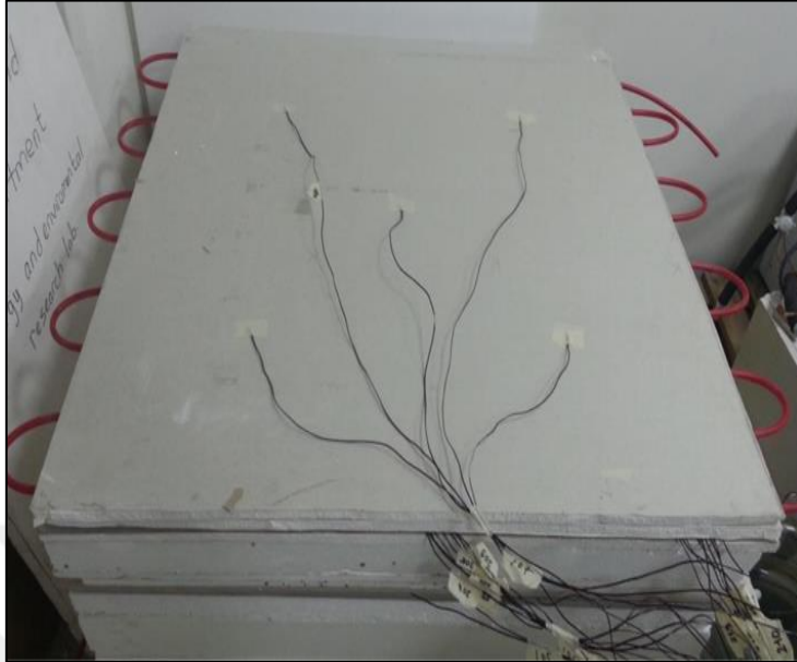
Figure 3.16 Thermocouples placed on the heat transfer plate.
