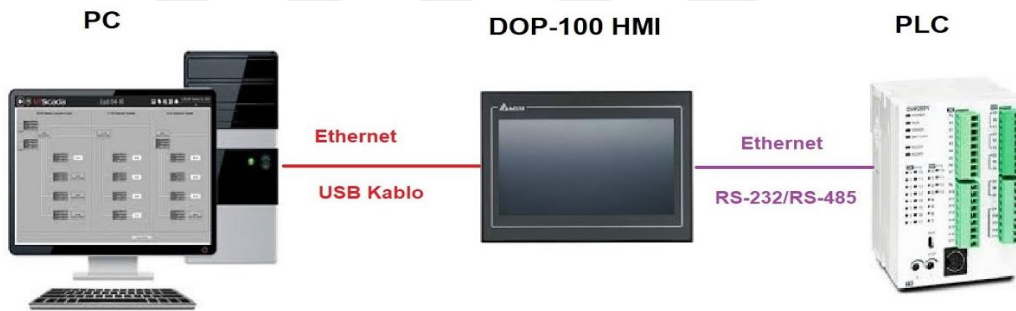
Figure 3.24 System working principle diagram
