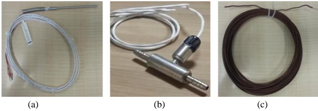
Figure 3.11 Sensors used for temperature measurement (a) RTD sensor, (b) PT100 for water temperature, (c) T-type thermocouple for surface temperature.
