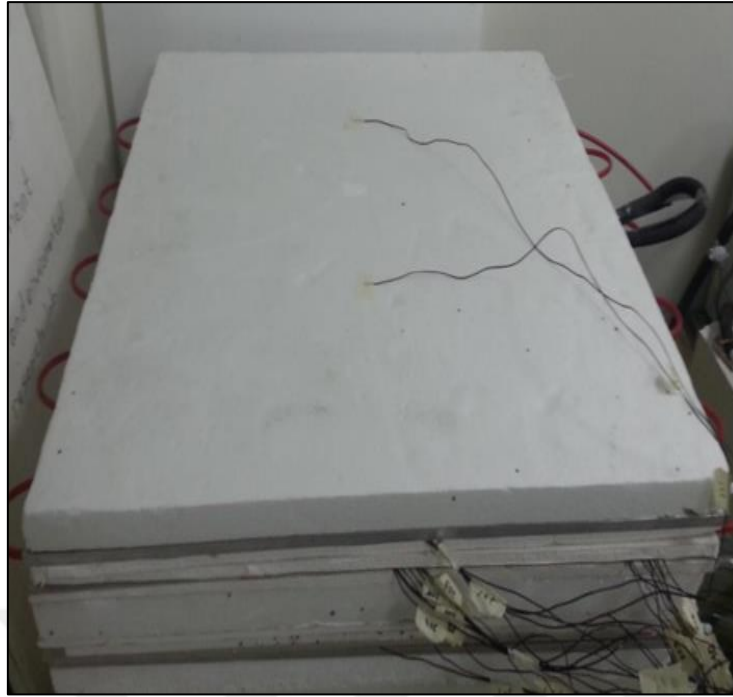
Figure 3.18 Thermocouples placed to measure the air temperature in the experimental setup.
