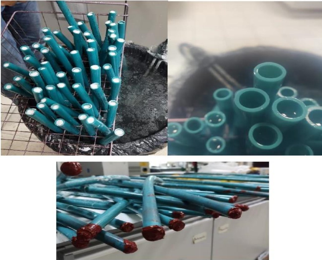
Figure 3.4 Macrocapsule tube filling and tube sealing process.
