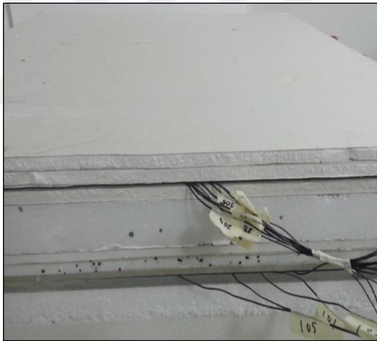
Figure 3.15 Cross-sectional view of the heat transfer layer placed on the hybrid wall sample.
