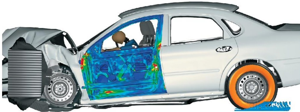
Figure 3.6. Abaqus/Explicit crash simulation of a car.
