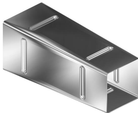
Figure 1.6. Rectangular cross-sectional tapered crash tube with double groove stamp.
