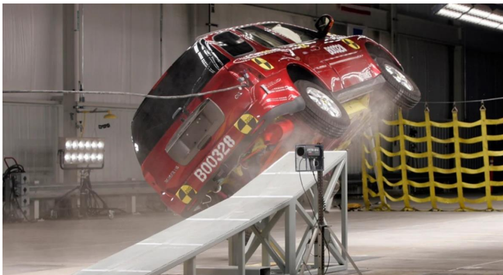
Figure 1.13. Roll over collision of the test car.
