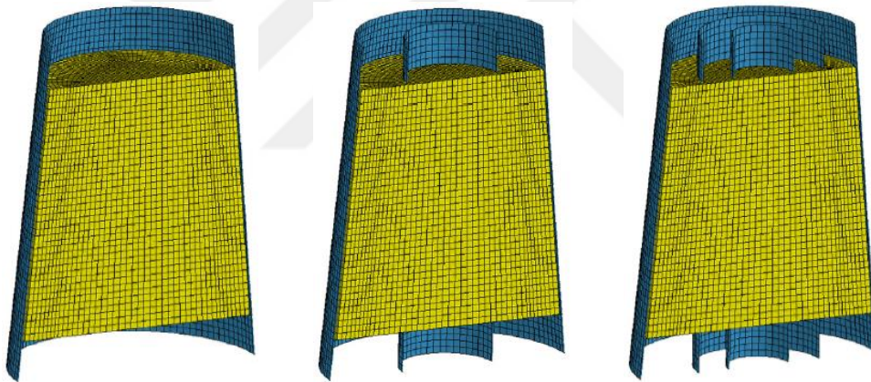
Figure 2.10. Mono-tubular (left), bi-tubular (middle), and tri-tubular axial foam-filled circular tubes with different foam heights [22].
