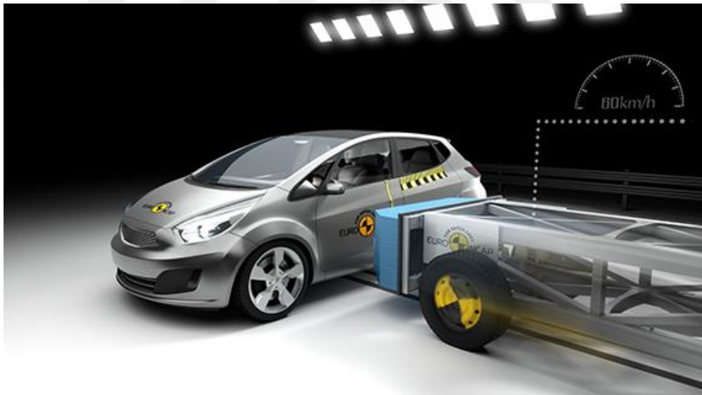
Figure 1.11. Lateral collision test between test car and deformable barrier.
