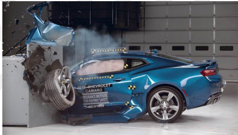
Figure 1.8. Frontal collision test of Chevrolet Camaro.
