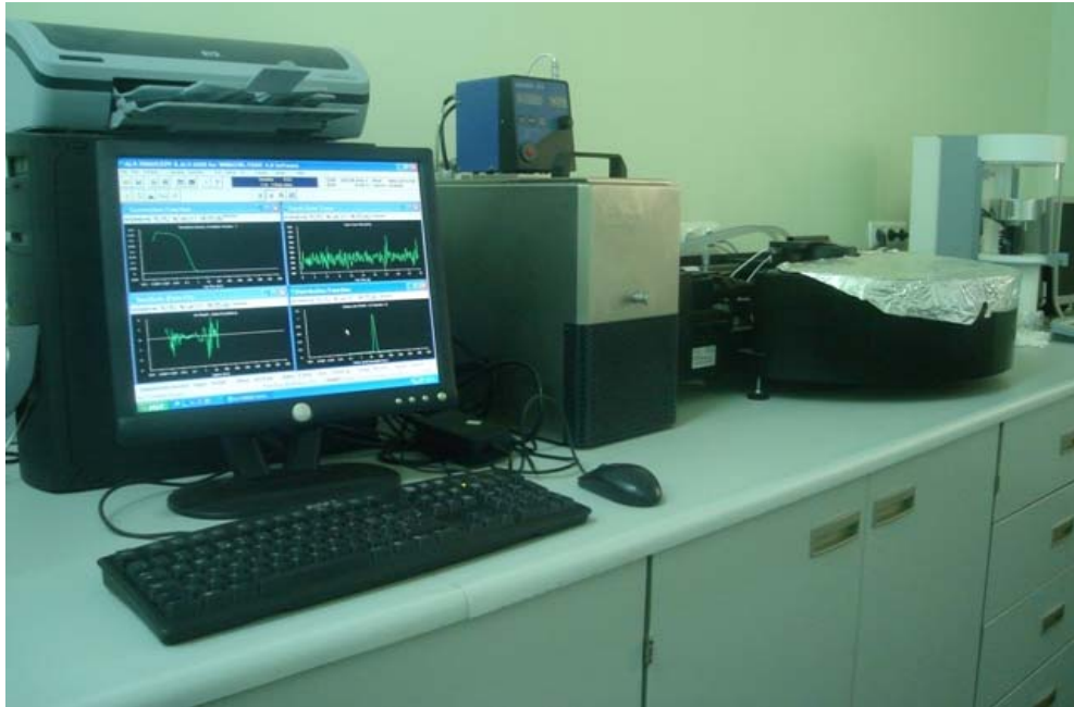
Şekil 4.54: DLS-SLS: ALV \ CGS 3 Compact Goniometer System
