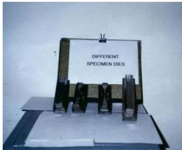
Figure 4.5 Dies used for cutting the sample for certain tests
