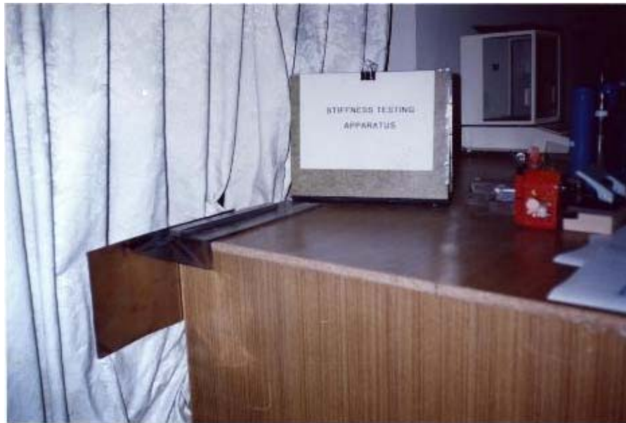
Figure 4.2 Apparatus for stiffness test on geomembrane.
