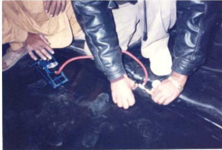
Figure 4.7 Pressurized dual seam technique (air pressure test)
