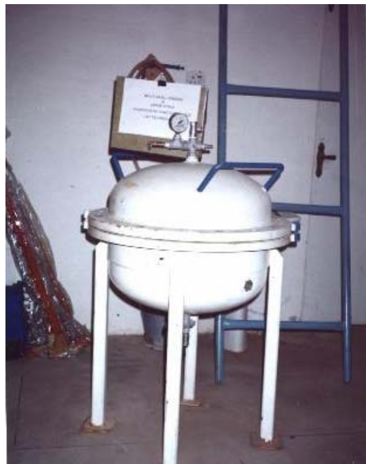
Figure 4.4 Hydrostatic puncture test for geomembrane
