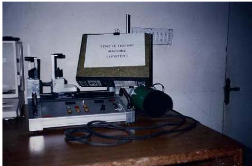
Figure 4.6 Tensile compression machine for tensile and seam tests.
