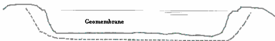
Figure 5.3 Geomembrane on the bed only under soil cover with no geotextile
