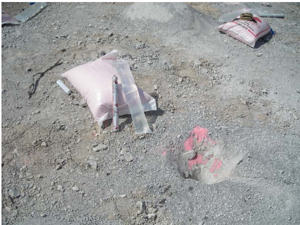
Figure 6.7 Production blast hole with 89mm diameter, ANFO, booster with detonator and a water deck (length of 50cm)
