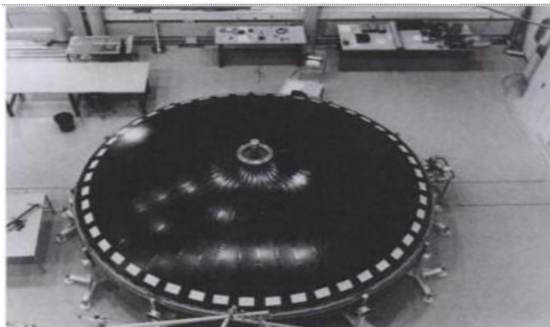
Figure 1.6: Inflatable very long baseline interferometry antenna, the 1980s. (Used under fair use, Ref. [3])
