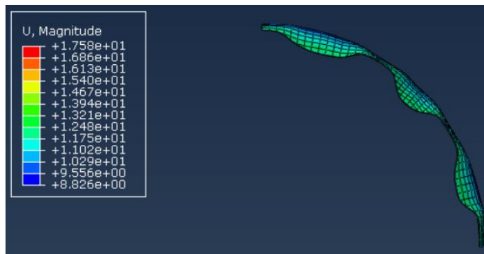
Figure 5.30: The drawn cup in the plane z = -5.5mm using the BBC2008-16p model
