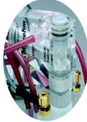
Multi-Mode Electrode ME - the time-proven all-purpose electrode
