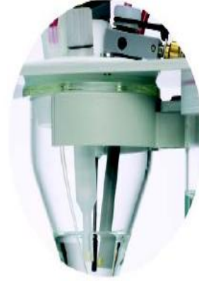
Rotating disk electrode (RDE) can be used in the same stand.
