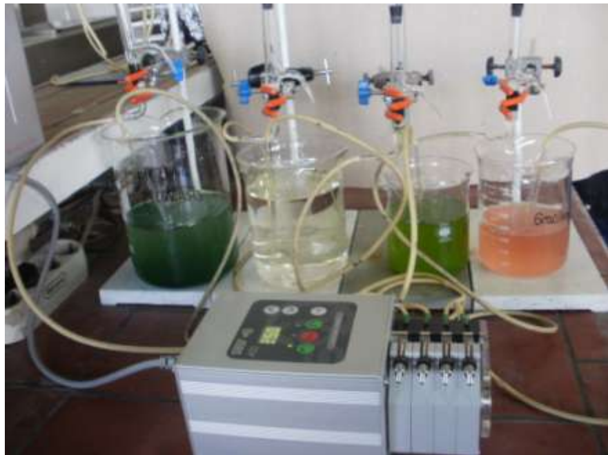
Figure 3.9 Biological contamination load to the continuous system
