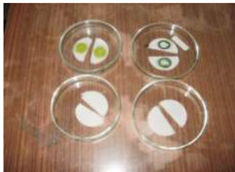
Figure 3.12 The filter papers with the dry weight of microorganisms on them
