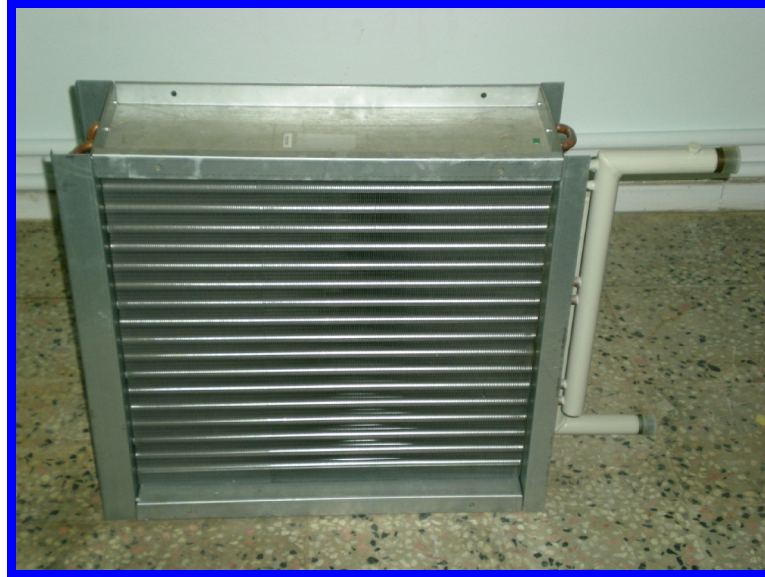
Figure 3.5. Picture of the cooling coil used
