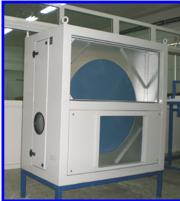
Figure 3.3. Picture of the desiccant wheel used
