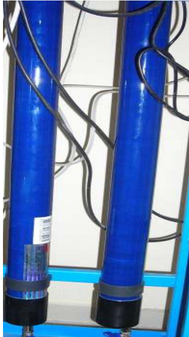
Figure 2.7 Spiral wound BWRO membranes
