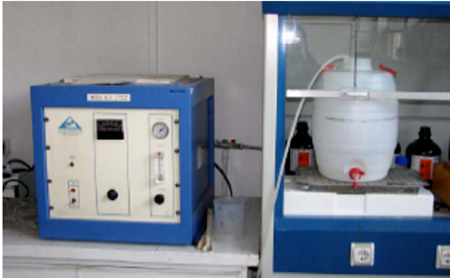
Figure III.2 Ozone Generator and Contact Unit
