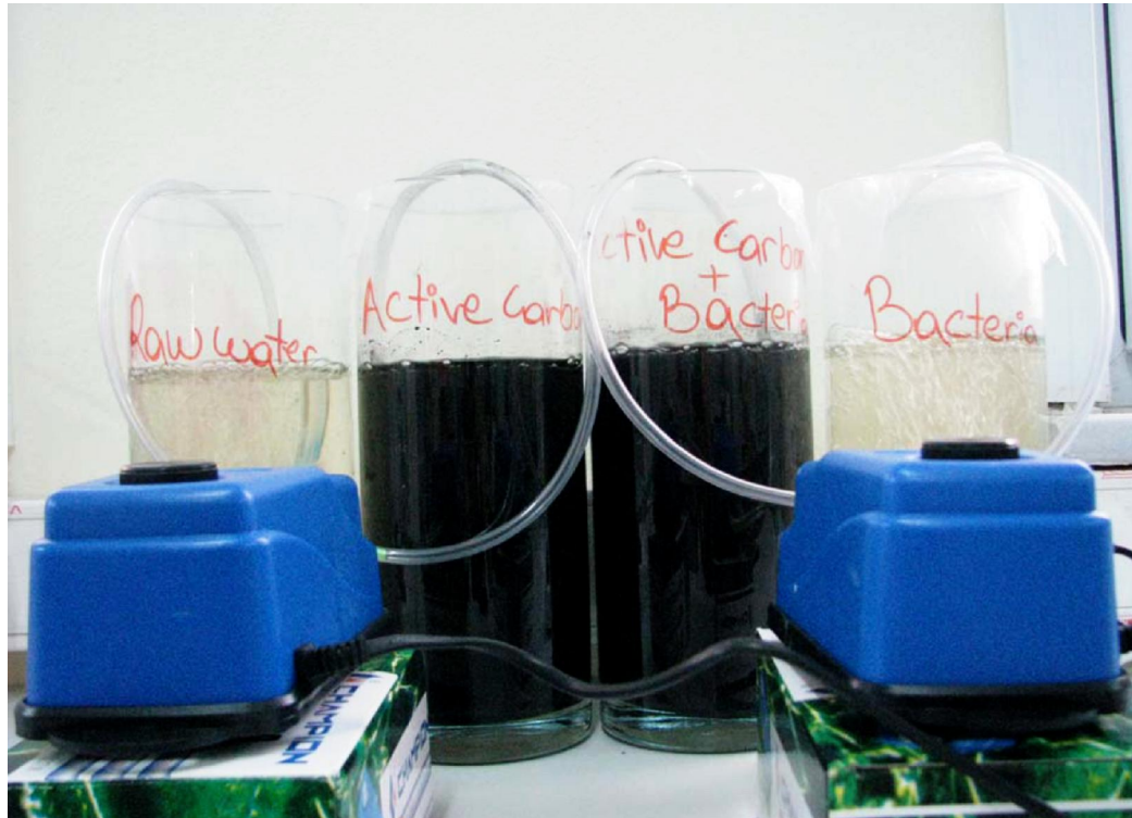
Figure III.3 Powdered Activated Carbon + Activated Sludge Reactors
