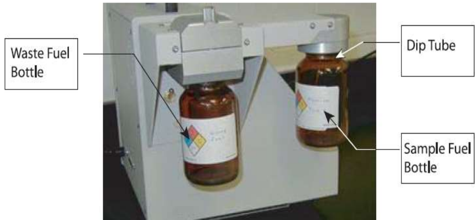
Figure 3.7 Standard sample run set-up
