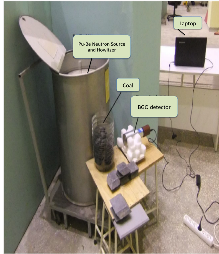
Figure 3.16 : The experimental set-up of Pu-Be neutron.
