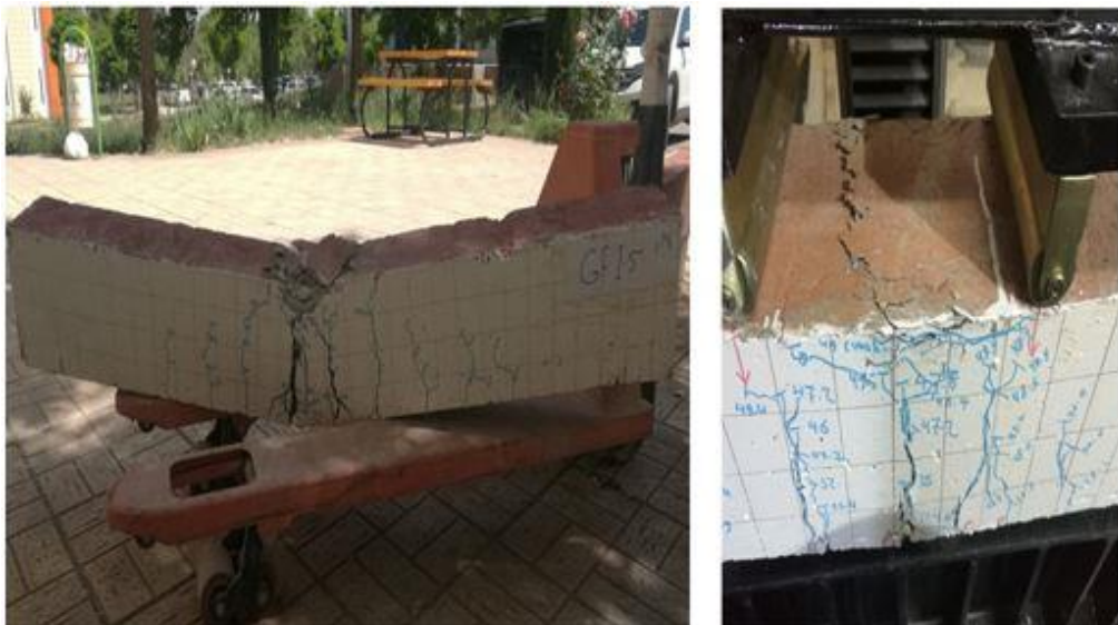
Figure 4.13 Beam A 3 GF after the crush and indicate crack propagation
