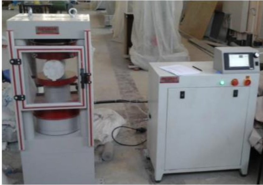
Figure 3.13 Compressive machine test for split tensile strength test
