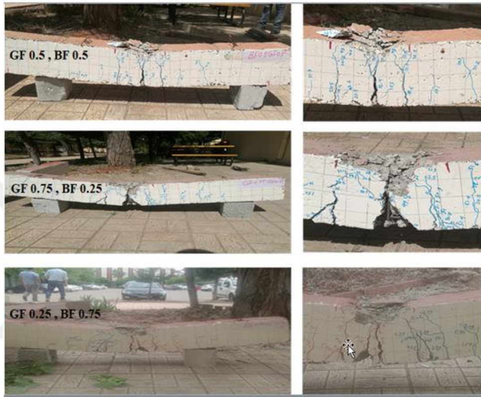
Figure 4.20 Flexural tests of Group C beam
