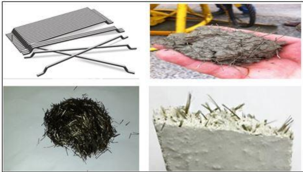
Figure 0.2 Steel and basalt fibers in the concrete
