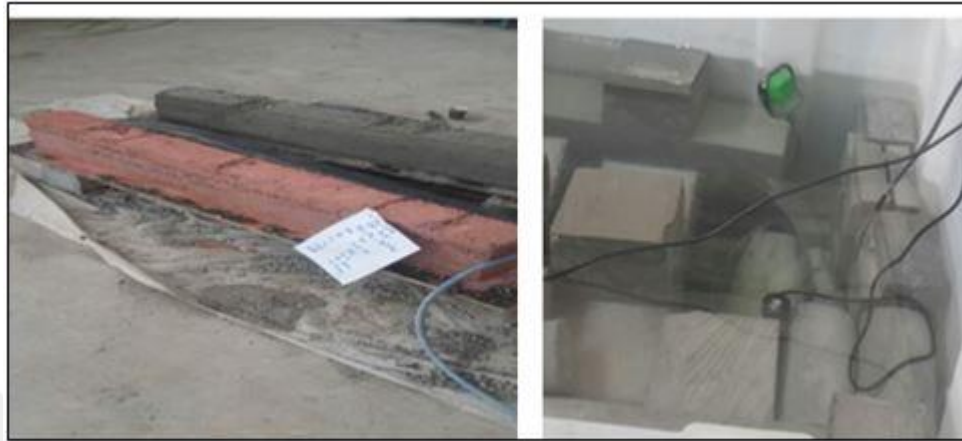
Figure 3.10 Curing of Samples and beams by the pool and members curing method
