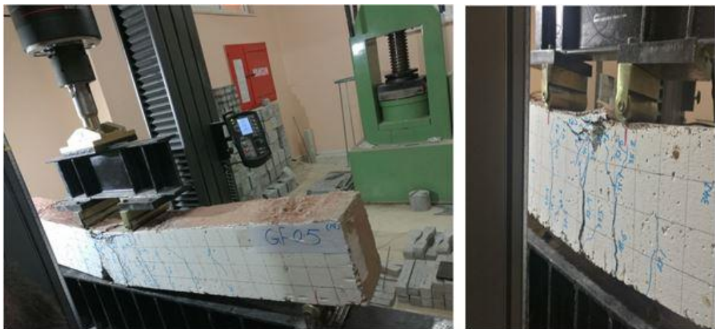
Figure 4.10 Flexural tests for concrete beam A 1 GF
