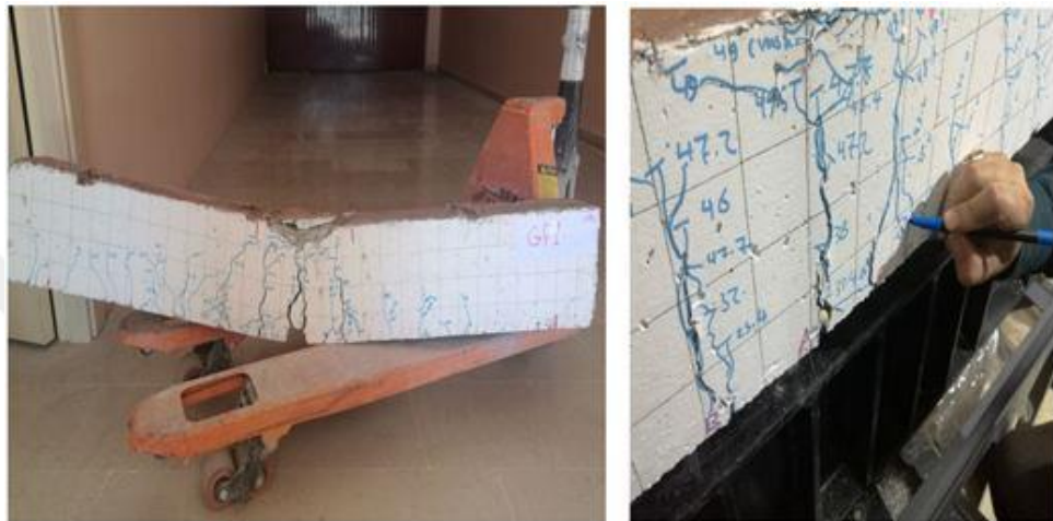
Figure 4.11 Beam A 2 GF after the crush and indicate crack propagation
