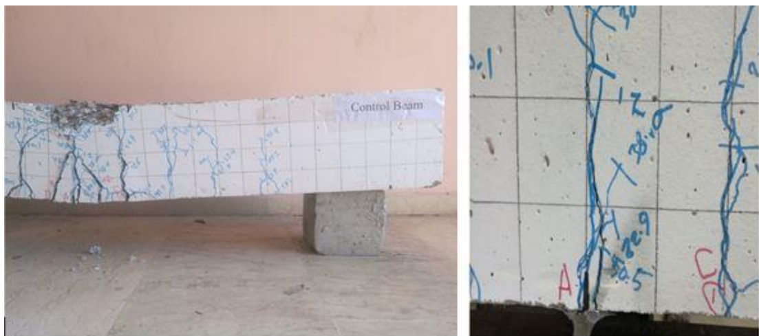
Figure 4.7 Control beam after the crush and indicate crack propagation
