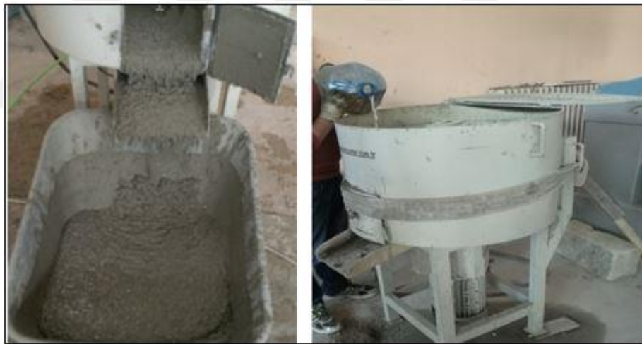
Figure 3.7 Proportioning, mixing and casting of beam specimen
