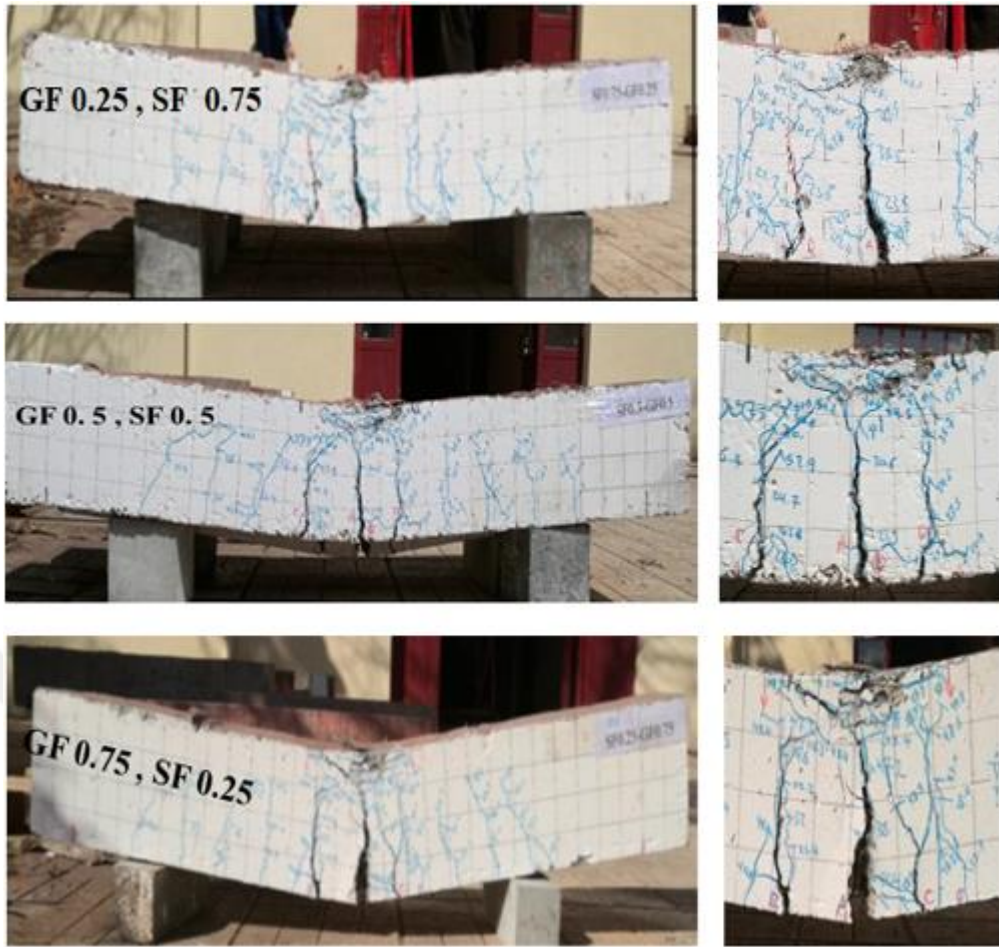
Figure 4.17 Result of Flexural test for Group B beams
