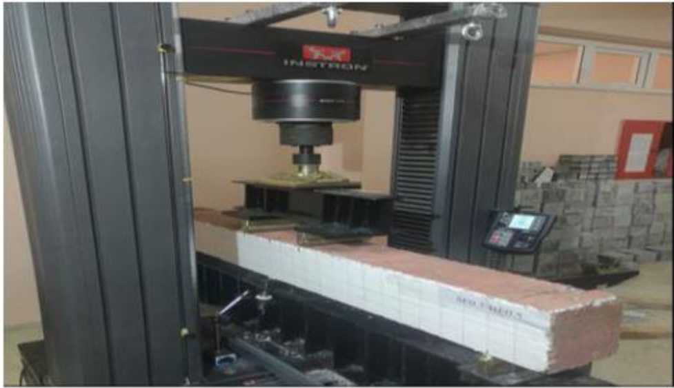
Figure 3.14 Flexural strength test machine for beams 4-point
