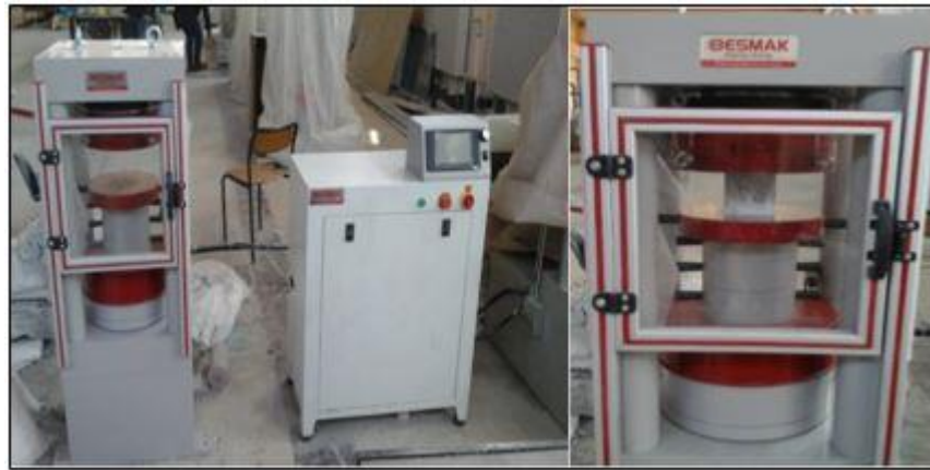
Figure 3.12 Compressive machine test for compressive strength test
