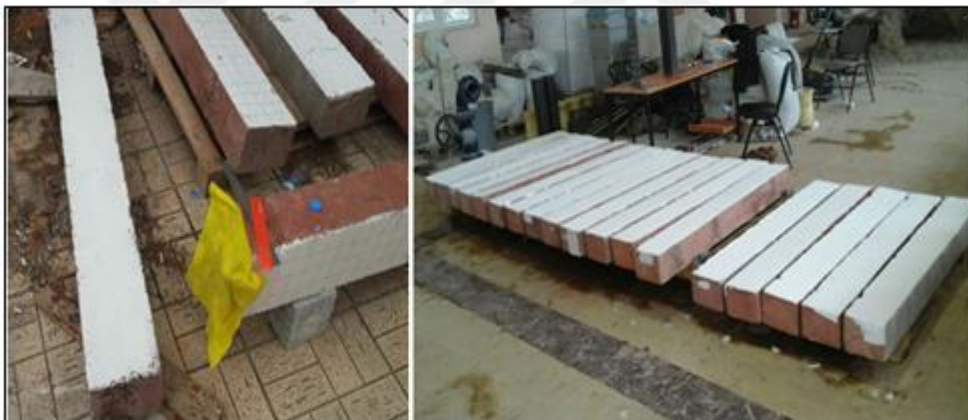
Figure 3.11 Preparation beams for flexural test
