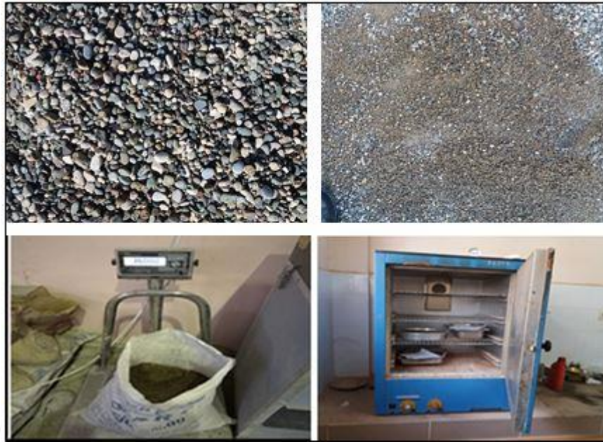
Figure 3.5 Drying process of the aggregates in furnace
