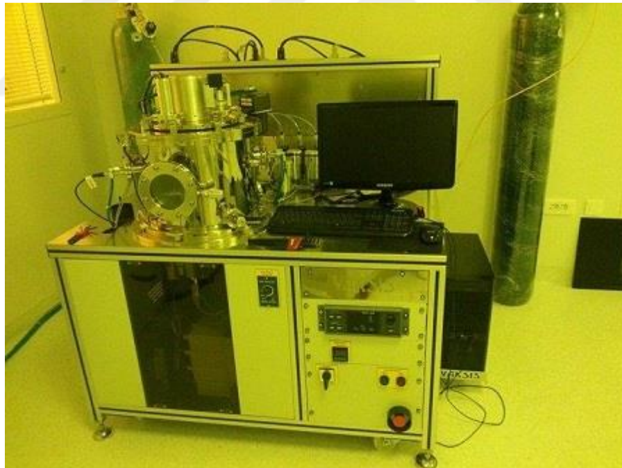
Figure 2.11: The magnetron sputtering system used for metal coatings.
