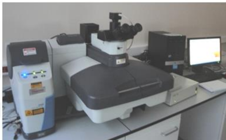
Figure 2.4: Raman Spectroscopy system (DXR, Thermo) used for graphene analysis.
