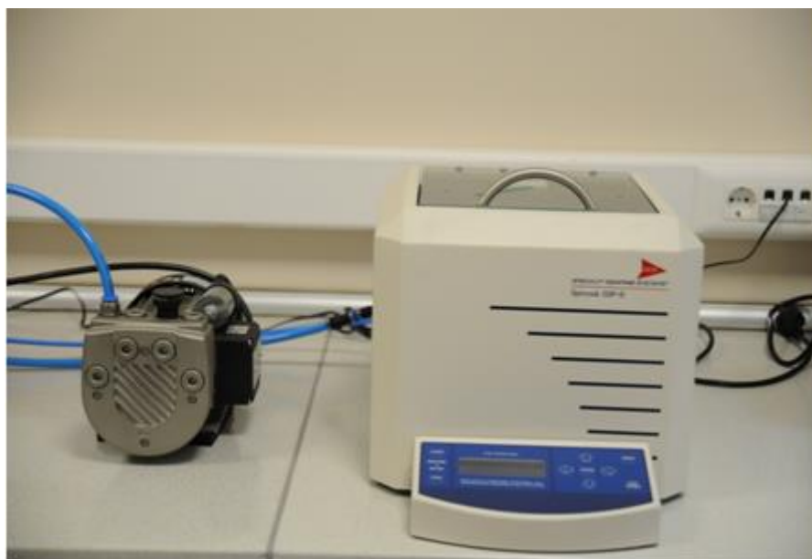
Figure 2.13: Spin-coater used for coating resists on wafers.
