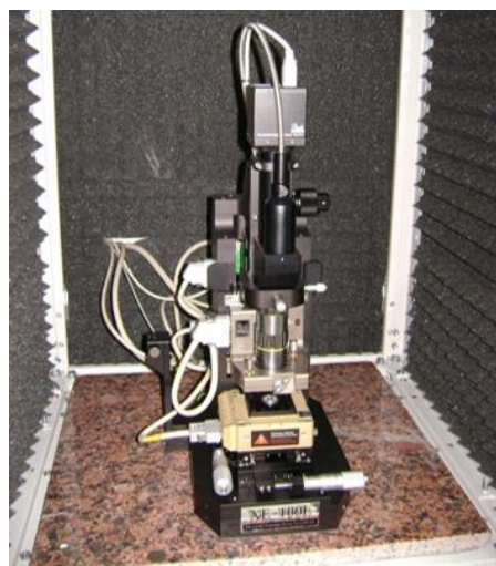
Figure 2.17: Atomic force microscopy system (XE-100, Park Systems).
