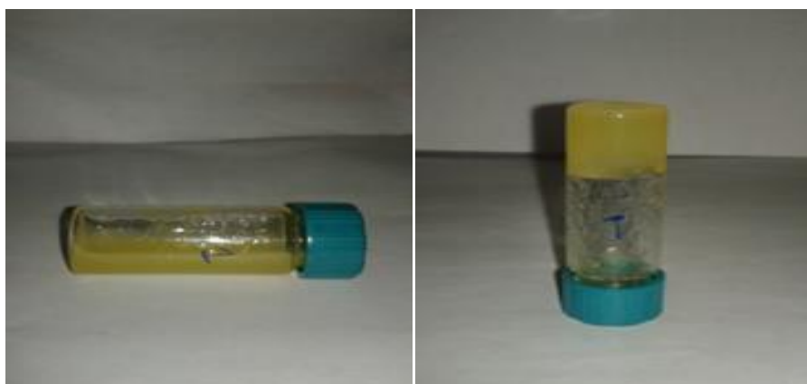
Figure 2.5 Photographs show liquid mixture of CF and bismaleimide (left) and cross-linked gel of Diels-Alder reaction (right).
