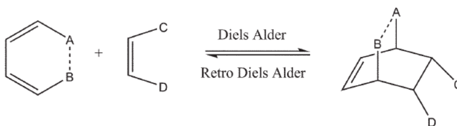
Figure 1.18 Diels-Alder Reaction Mechanism (Bergman & Wudl, 2008).
