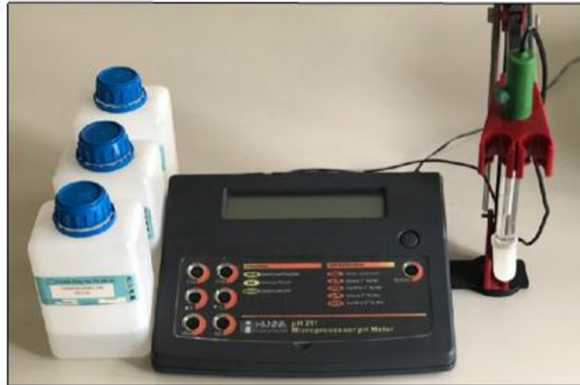
Şekil 3.16: pH Metre, Hanna Instruments pH211 Microprocessor.
