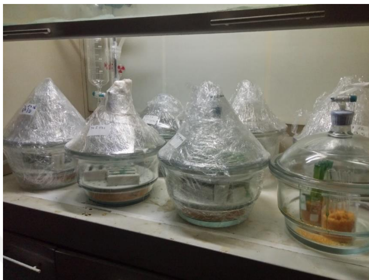
Figure 2.8 : Moulds were placed inside vacuum desiccators inside a glove bag and sealed with polymer industrial polypropylene.
