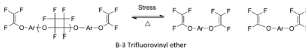
Figure 1.17 : Mechanically induced chain cleavage in perfluoro-cyclobutane (Y. Yang & Urban, 2013)
