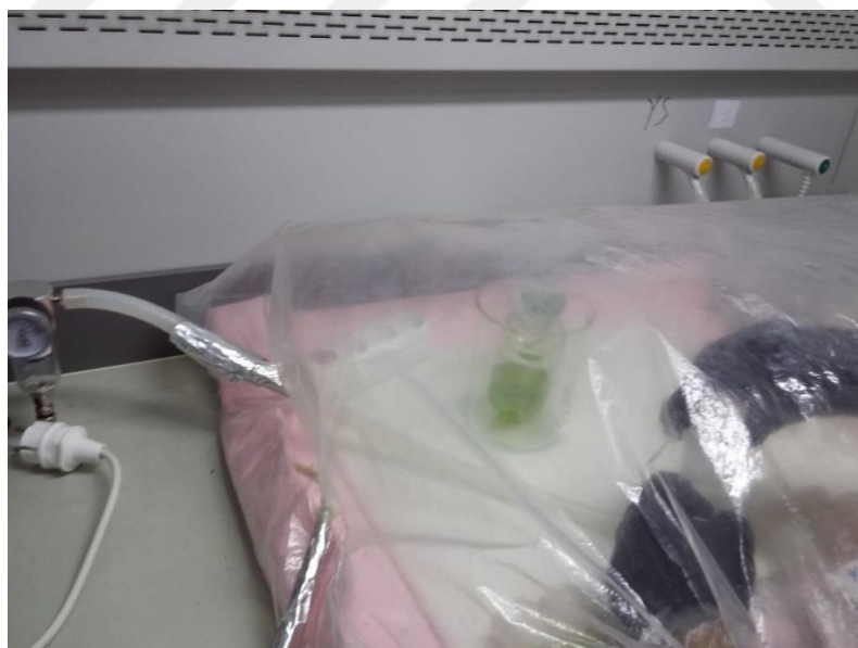
Figure 2.6 : An extra pure argon purge for 30 minutes.
