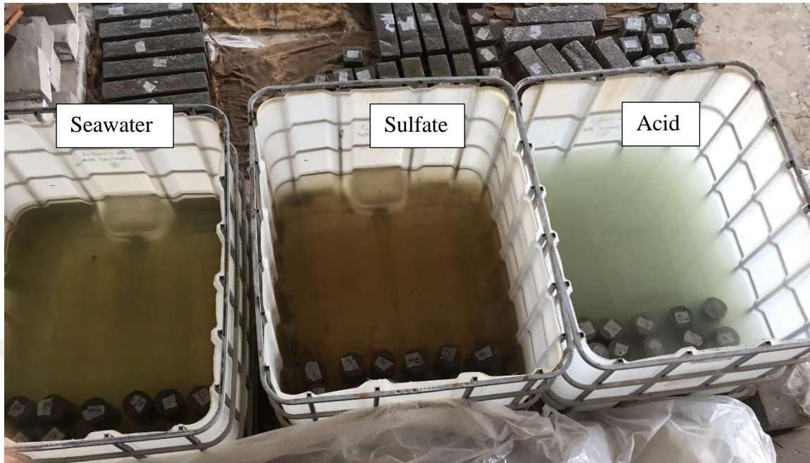
Figure 3.11 GPC and NC concrete specimens submerged in chemical attack
