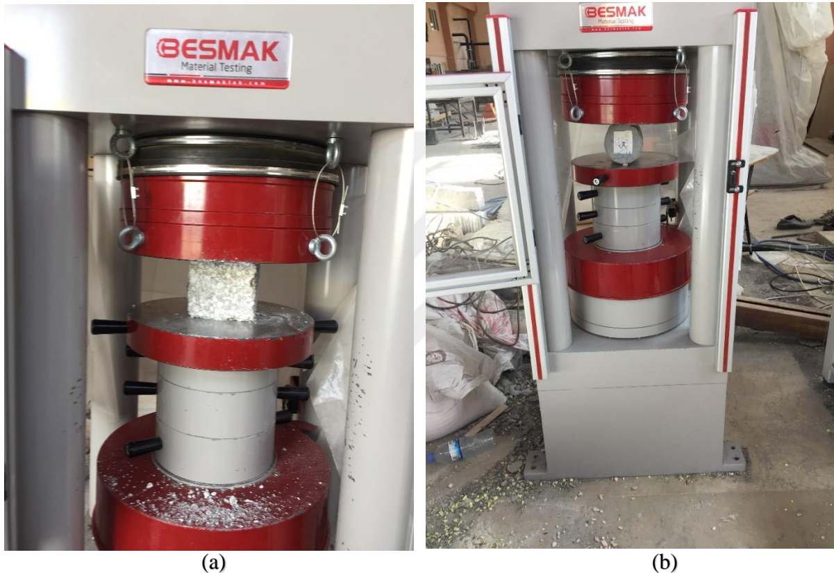
Figure 3.13 Strength test (a) compression test and (b) splitting tensile test
