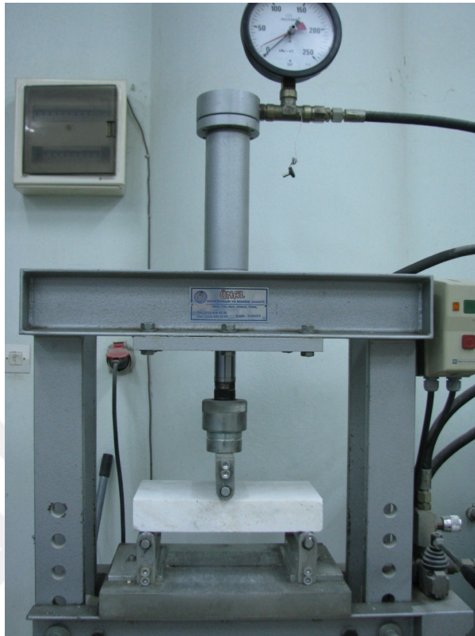
Figure 5.2 Practice of bending strength under heavy load
