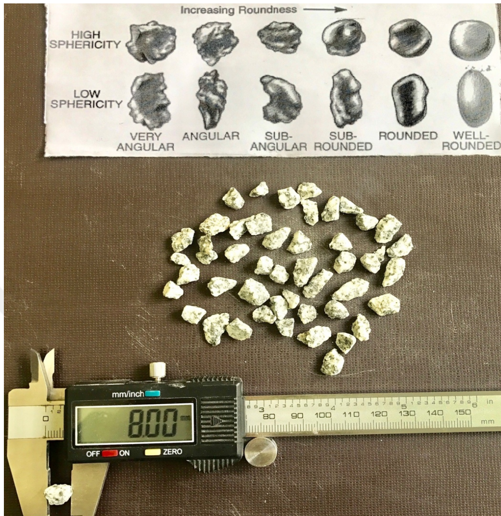
Figure 6.7 Granite aggregate with 4-8 mm grain size (Personal archive, 2017)
