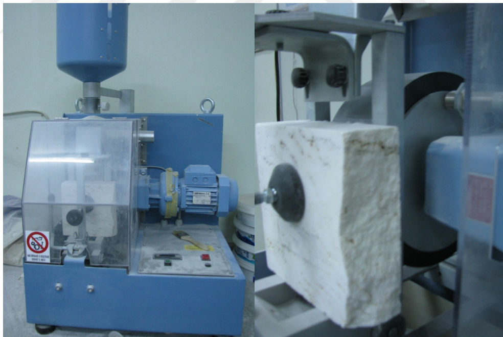
Figure 5.4 Abrasion resistance test with large disc
