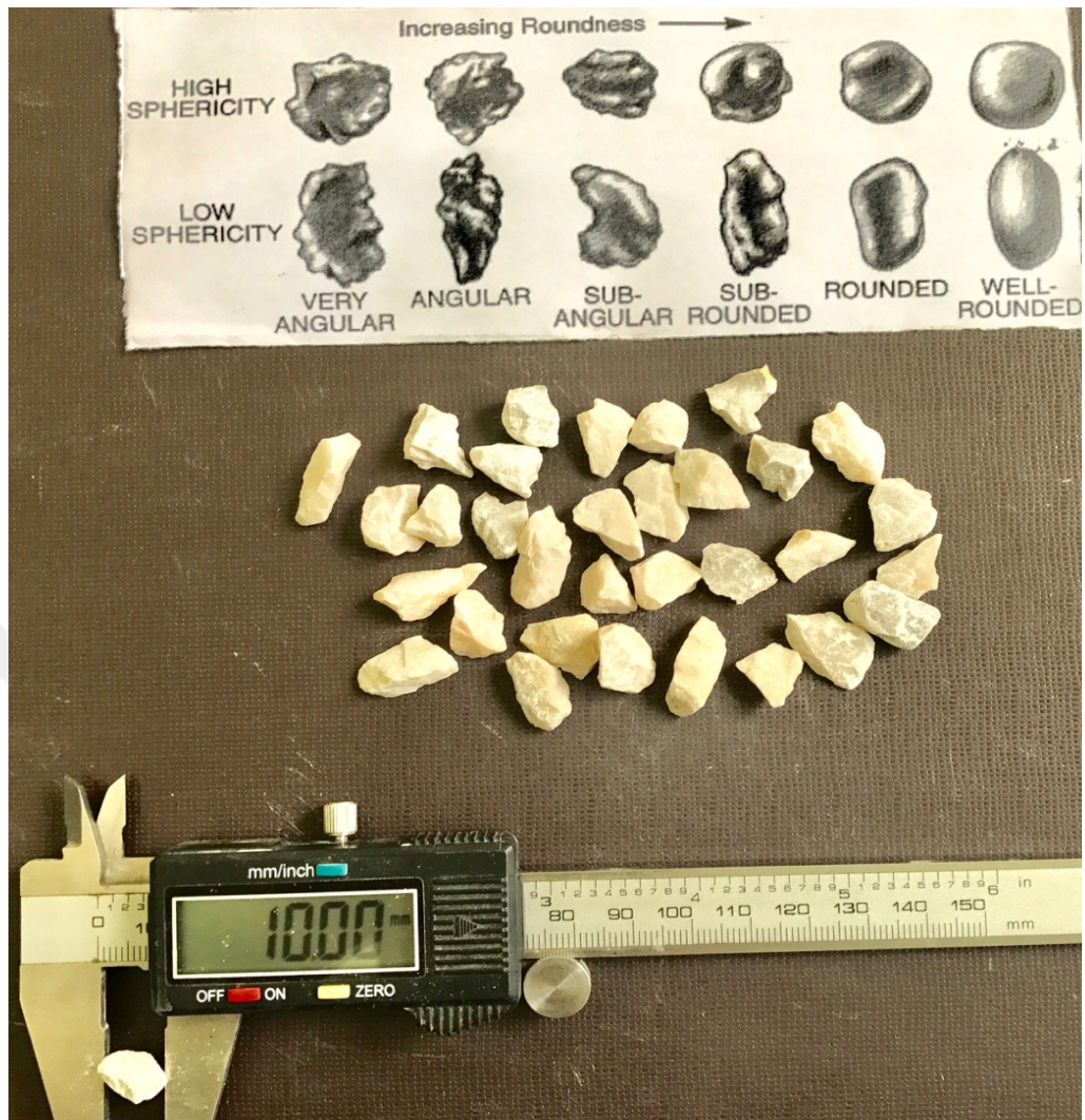
Figure 6.12 Limestone aggregate with 8-10 mm grain size (Personal archive, 2017)
