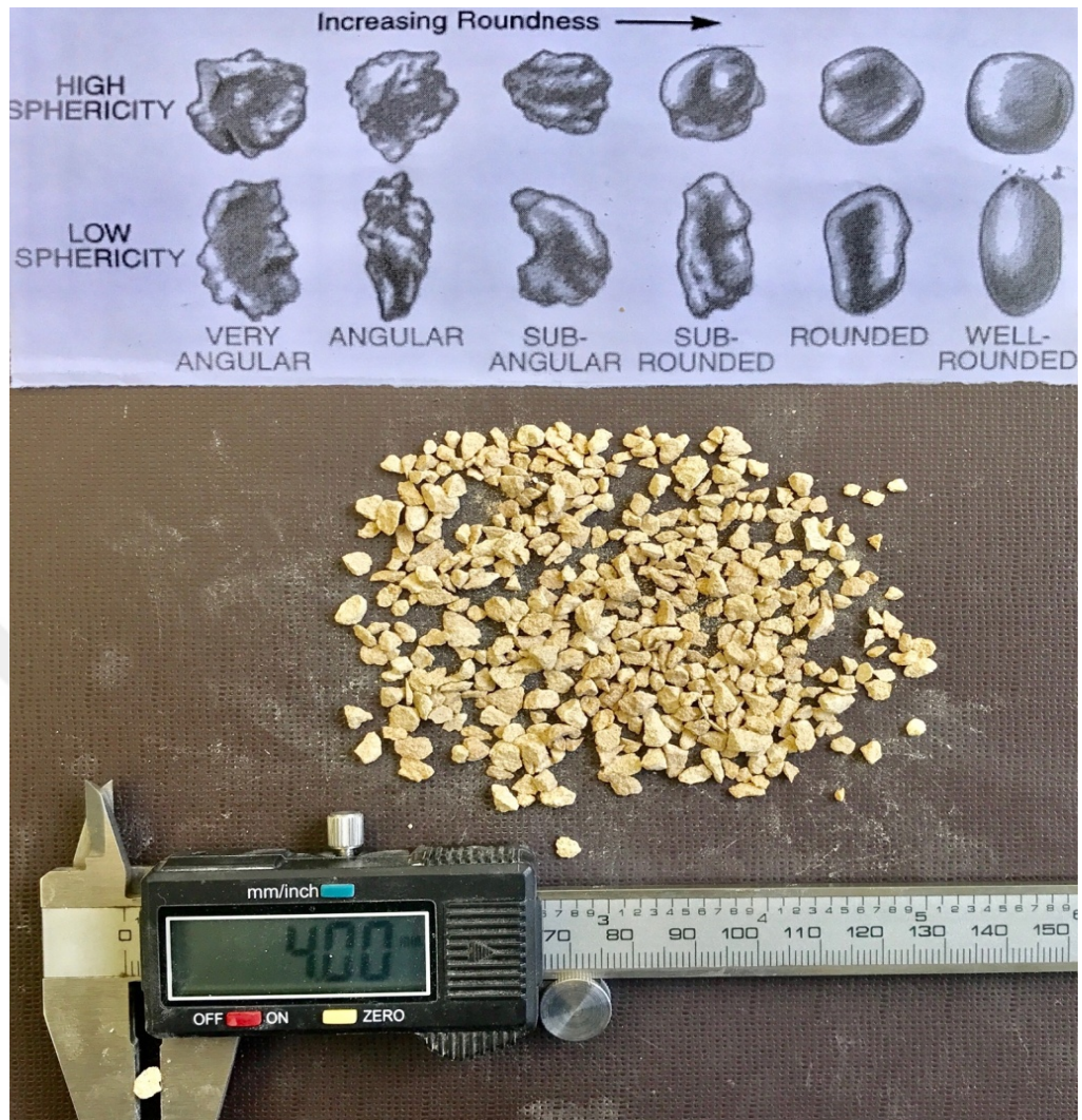
Figure 6.14 Sandstone aggregate with 2-4 mm grain size (Personal archive, 2017)
