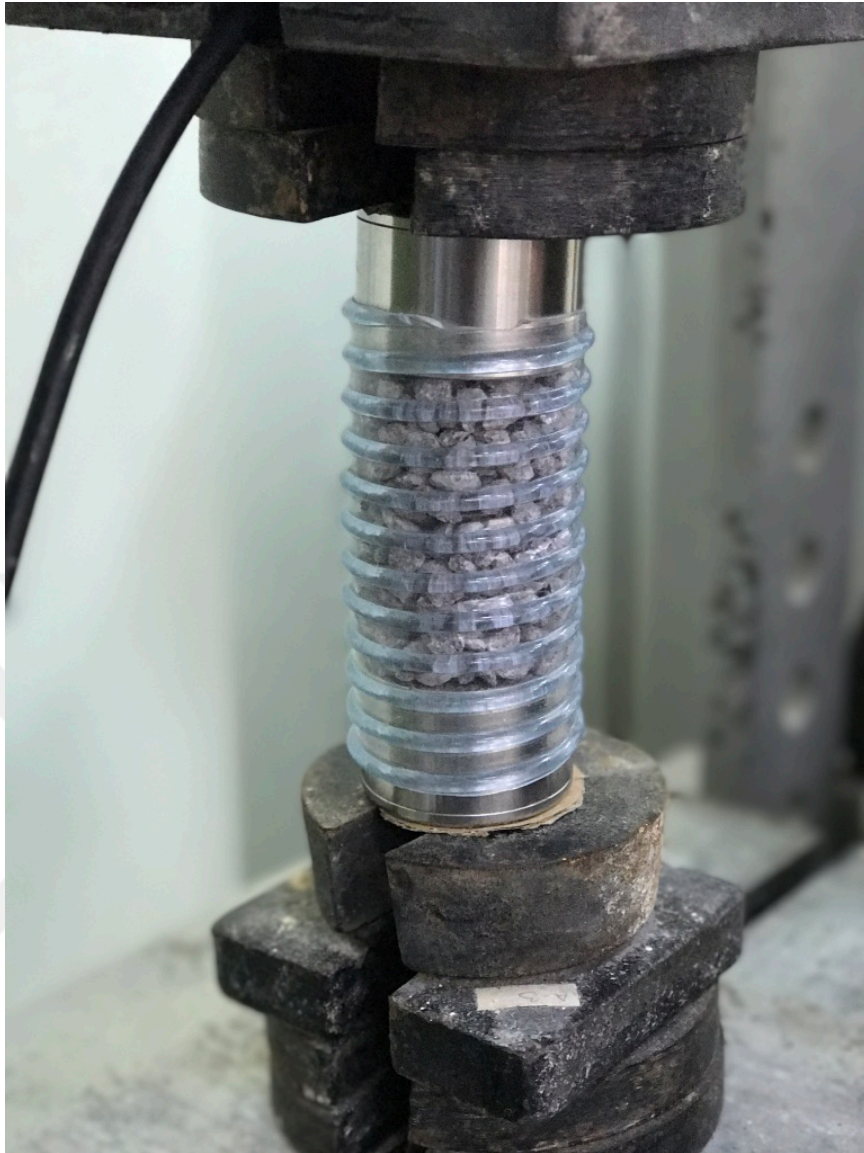
Figure 6.36 Andesite granular material inside the tube with ultrasonic probes at both ends (Personal archive, 2017)
