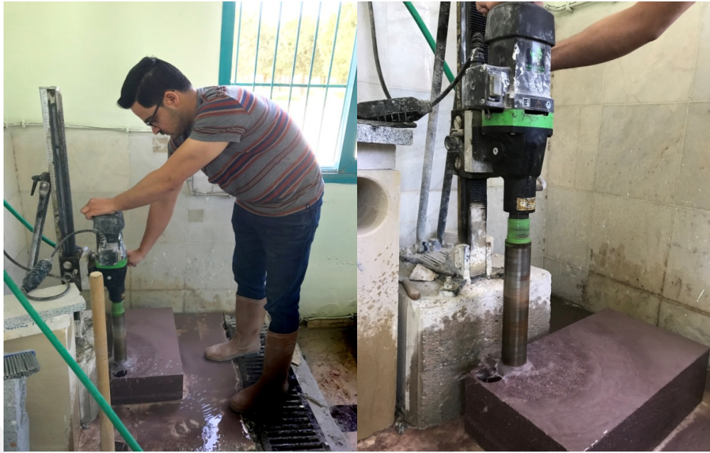
Figure 2.2 Core samples drilling from block (Personal archive, 2017)
