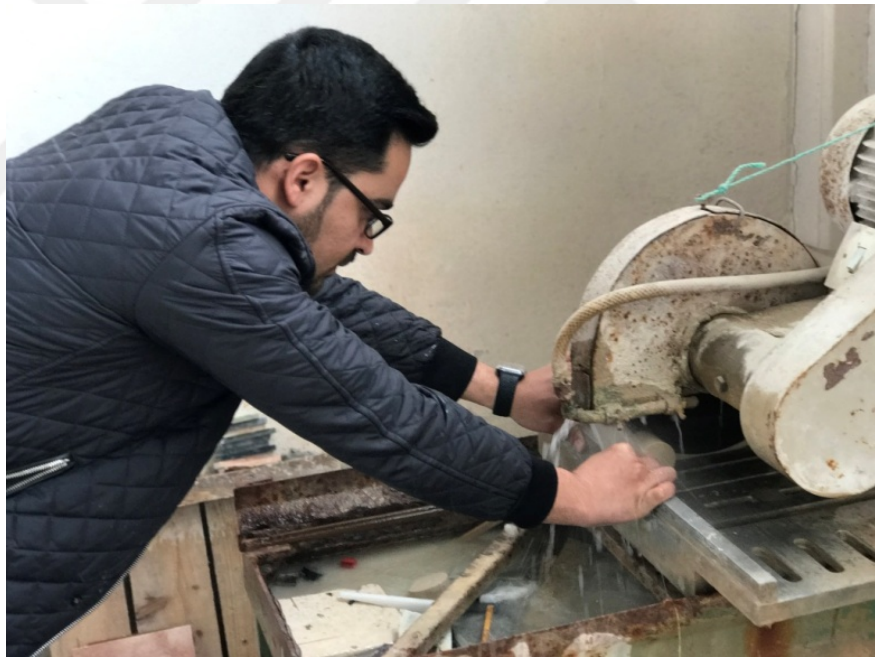
Figure 2.3 Cutting cores to desired diameter (Personal archive, 2017)
