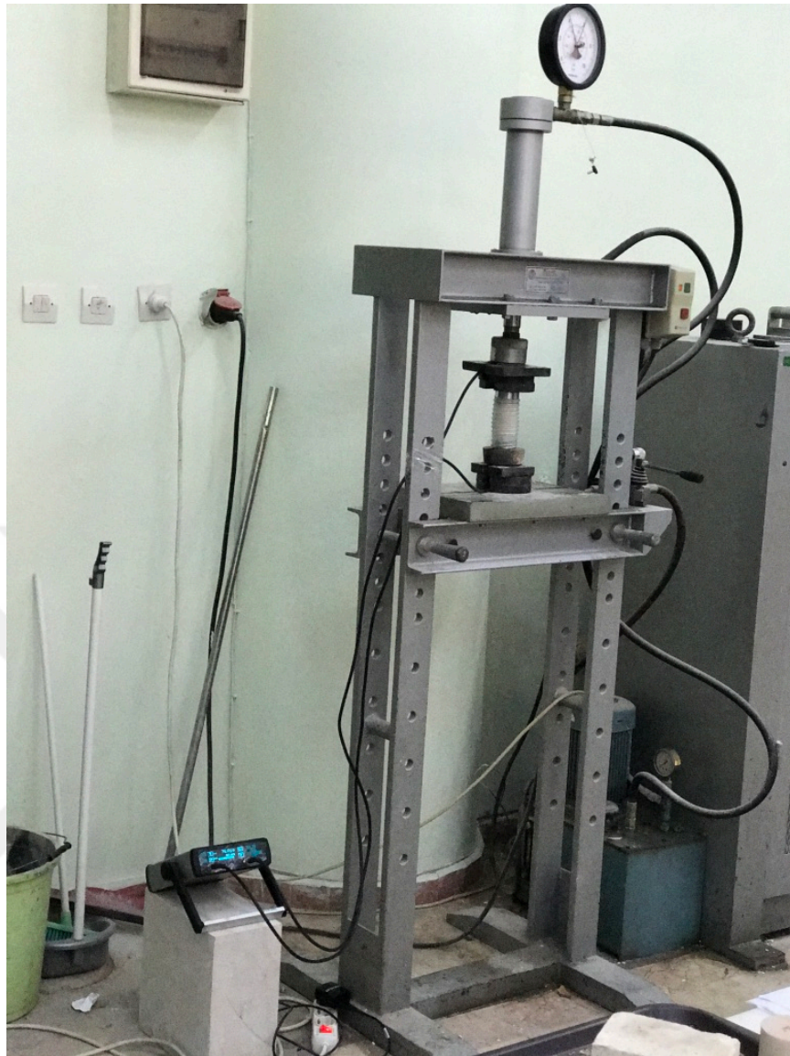
Figure 6.37 Laboratory setup for ultrasonic testing of granular materials (Personal archive, 2017)
