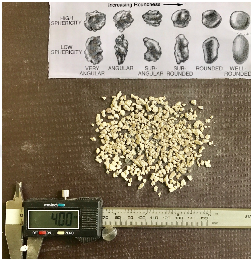
Figure 6.18 Tuff aggregate with 2-4 mm grain size (Personal archive, 2017)
