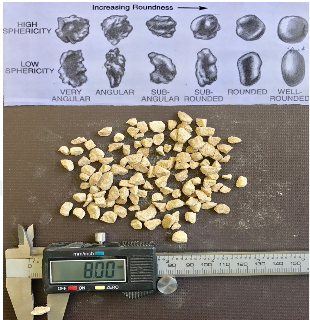
Figure 6.15 Sandstone aggregate with 4-8 mm grain size (Personal archive, 2017)
