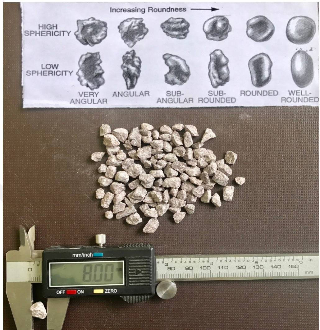
Figure 6.3 Andesite aggregate with 4-8 mm grain size (Personal archive, 2017)
