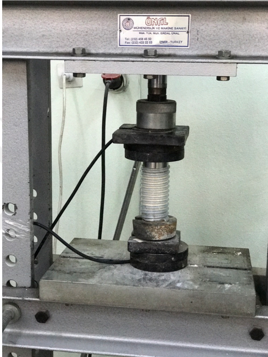
Figure 6.35 Compressing Tuff aggregate sample for ultrasonic test (Personal archive, 2017)
