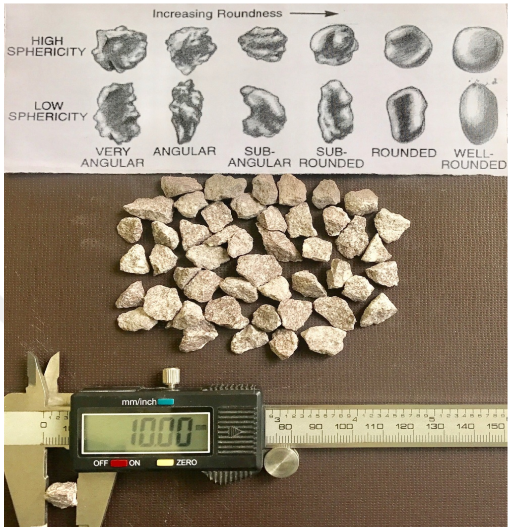
Figure 6.4 Andesite aggregate with 8-10 mm grain size (Personal archive, 2017)
