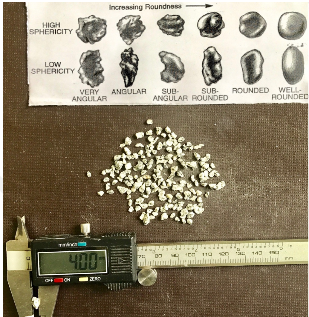
Figure 6.6 Granite aggregate with 2-4 mm grain size (Personal archive, 2017)
