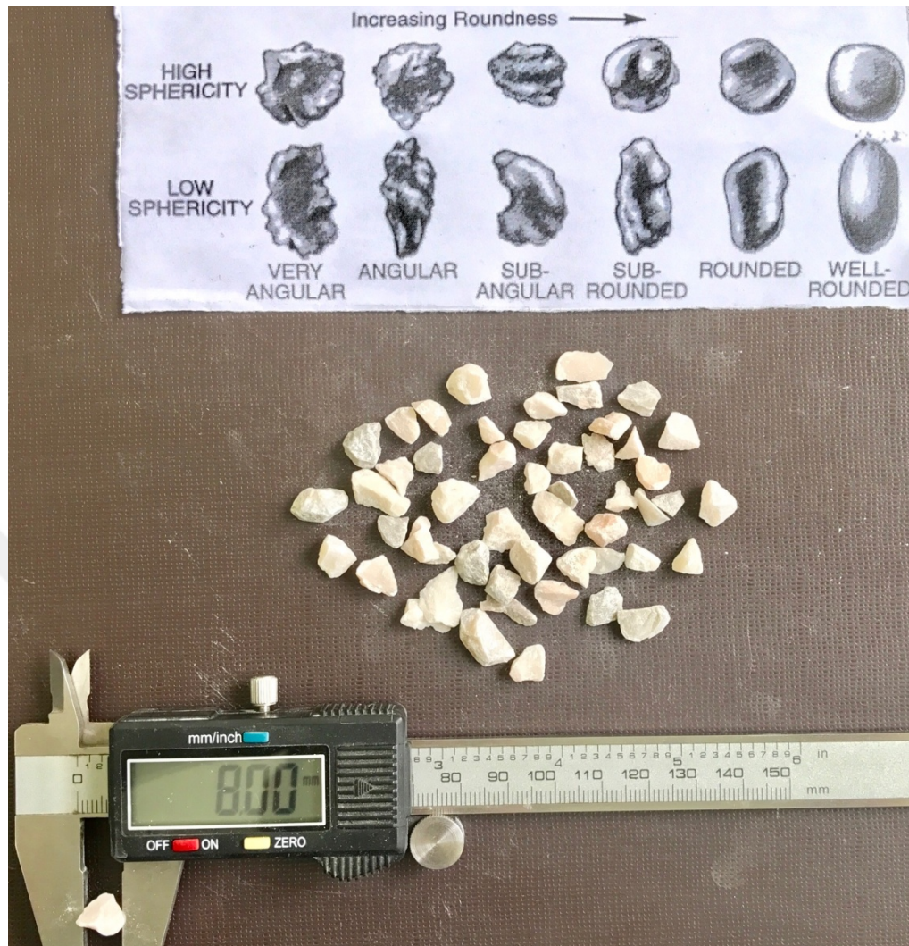
Figure 6.11 Limestone aggregate with 4-8 mm grain size (Personal archive, 2017)
