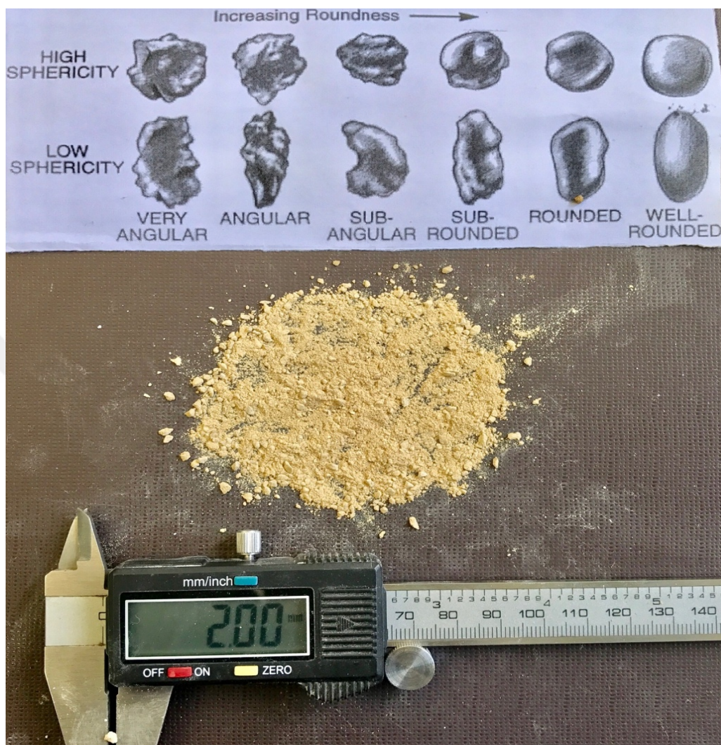
Figure 6.13 Sandstone aggregate with 0-2 mm grain size (Personal archive, 2017)
