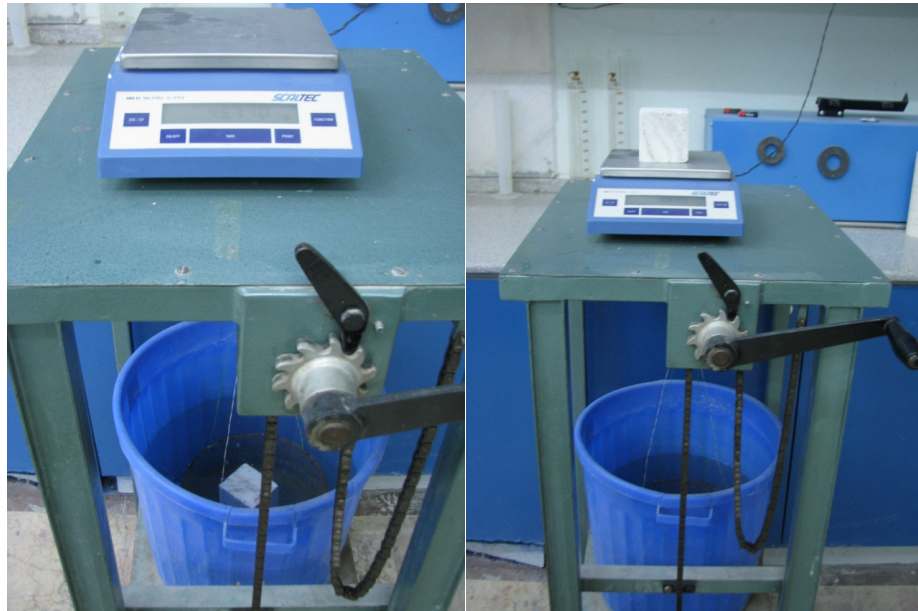
Figure 4.1 Samples measurements by Archimedes Balance (Personal archive, 2017)
