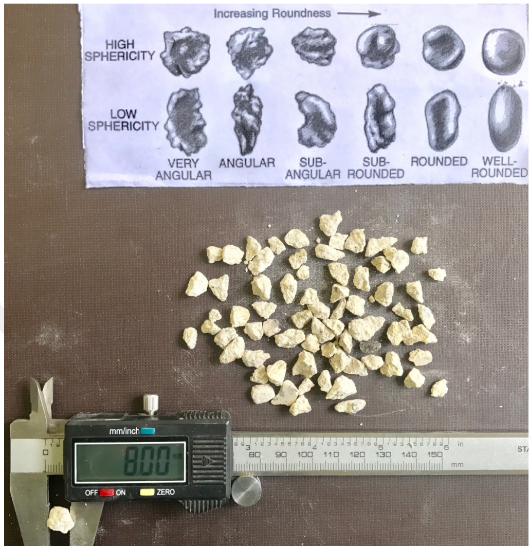
Figure 6.19 Tuff aggregate with 4-8 mm grain size (Personal archive, 2017)
