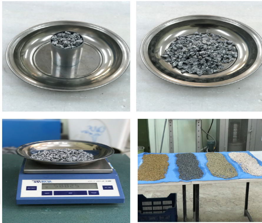
Figure 6.21 Dry and saturated bulk density measurement (Personal archive, 2017)
