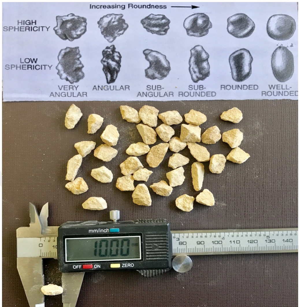
Figure 6.16 Sandstone aggregate with 8-10 mm grain size (Personal archive, 2017)
