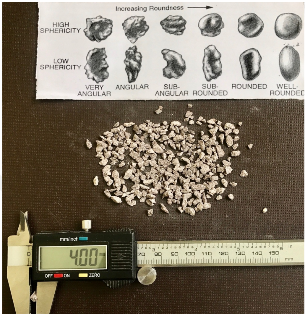
Figure 6.2 Andesite aggregate with 2-4 mm grain size (Personal archive, 2017)
