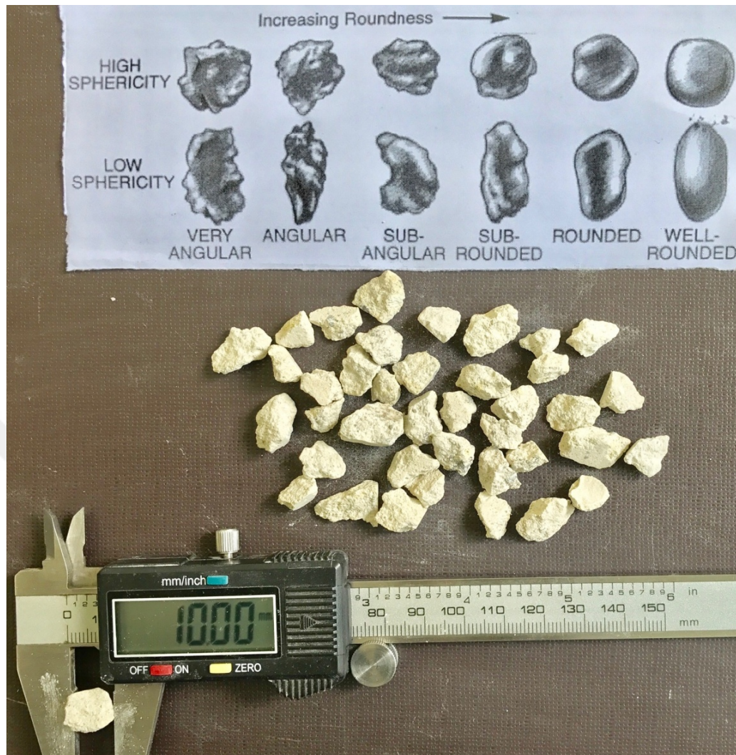
Figure 6.20 Tuff aggregate with 8-10 mm grain size (Personal archive, 2017)
