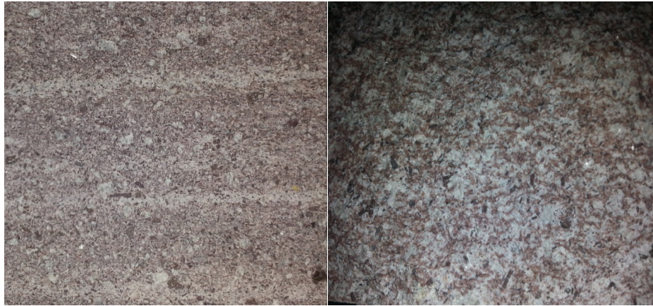
Figure 3.2 Macro photos display, a) lava-flow texture, b) fractured surface from the andesite sample
