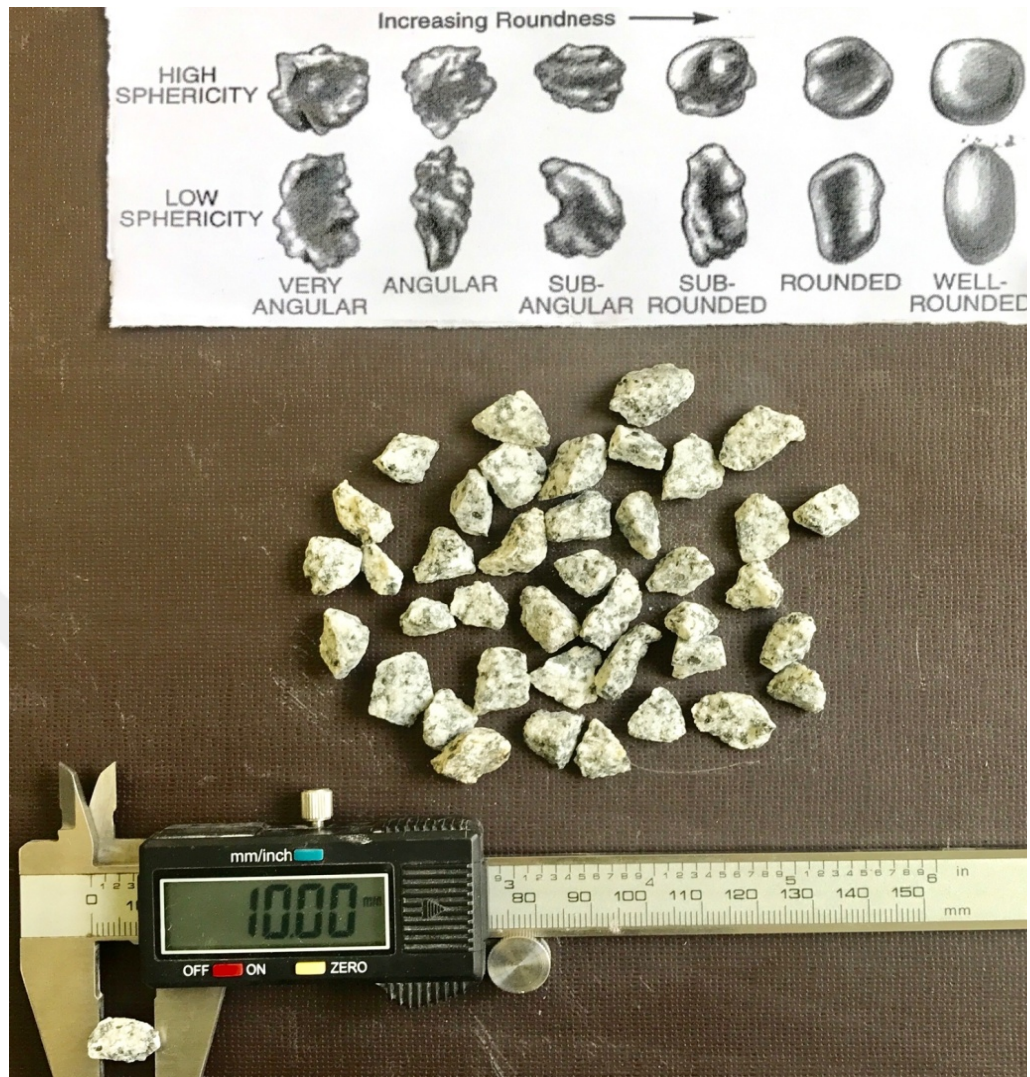
Figure 6.8 Granite aggregate with 8-10 mm grain size (Personal archive, 2017)
