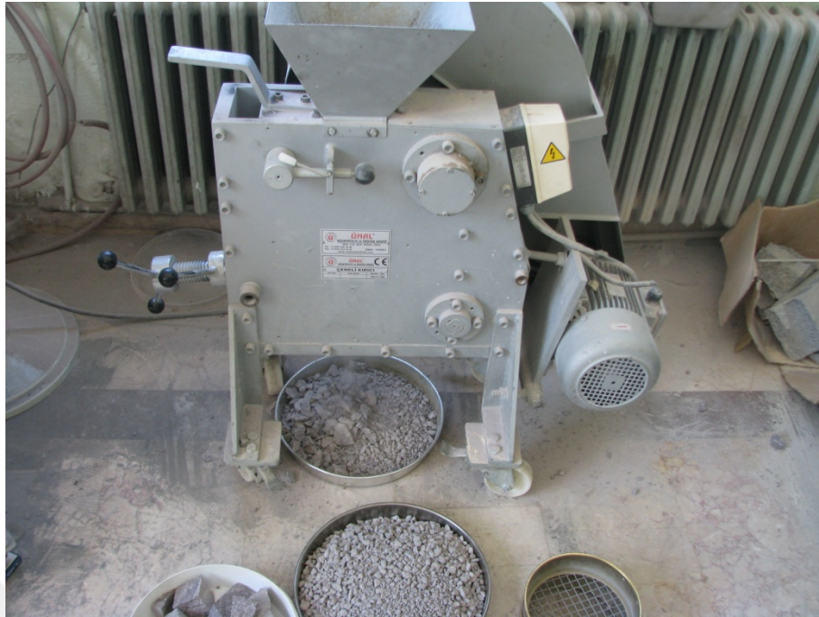
Figure 2.6 Preparation of aggregate samples (Personal archive, 2017)
